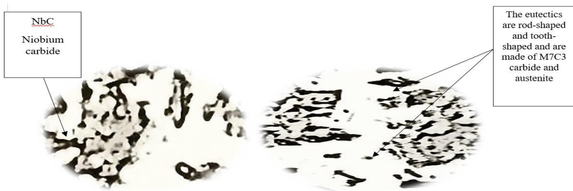
Fig. 9. Resulting microstructure of the first case sample, high-chromium white cast iron with 0.491% Nb and 2.75% Mn, after heat treatment 2.
