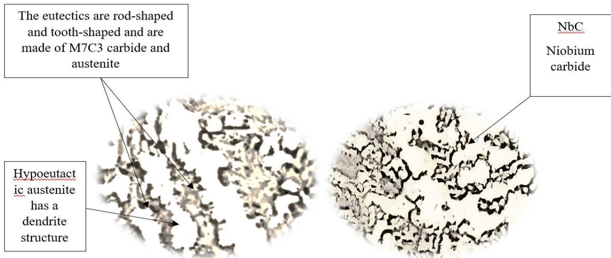
Fig. 7. Resulting microstructure of the first case sample, high-chromium white cast iron with 0.491% Nb and 2.75% Mn, without heat treatment.
