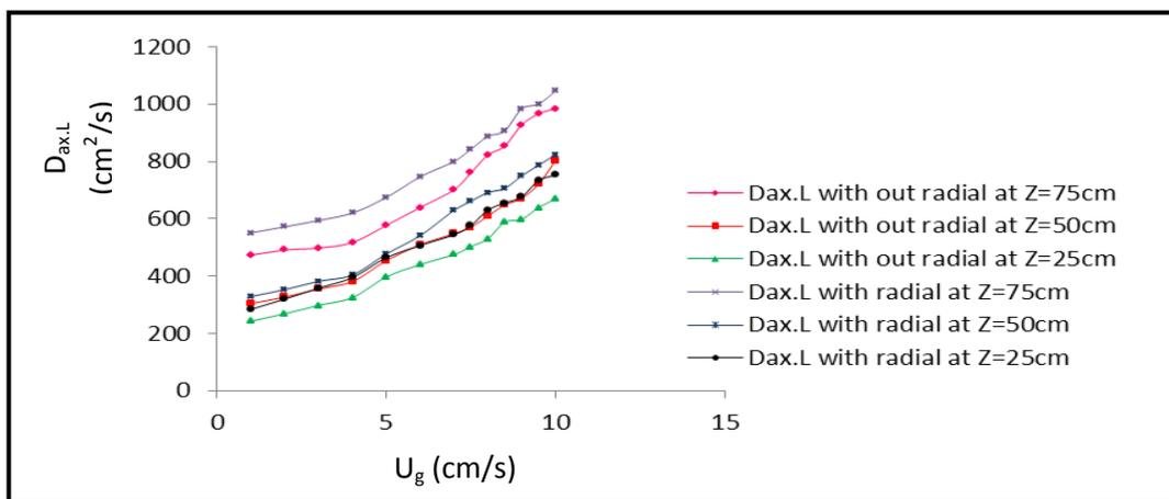
Fig. 4. Effect of Superficial Gas Velocity on Axial Liquid Dispersion Coefficient at Different Z,  $C_S=30$  and  $dp=3mm$ .
