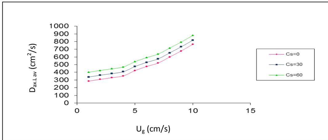
Fig. 11. Effect of Superficial Gas Velocity and Solid Concentration on Average Axial Liquid Dispersion Coefficient at dp= 1.5mm.
