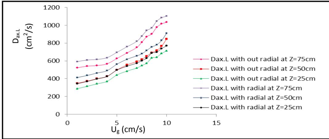
Fig. 6. Effect of Superficial Gas Velocity on Axial Liquid Dispersion Coefficient at Different Z, CS=30 and dp= 1.5mm.
