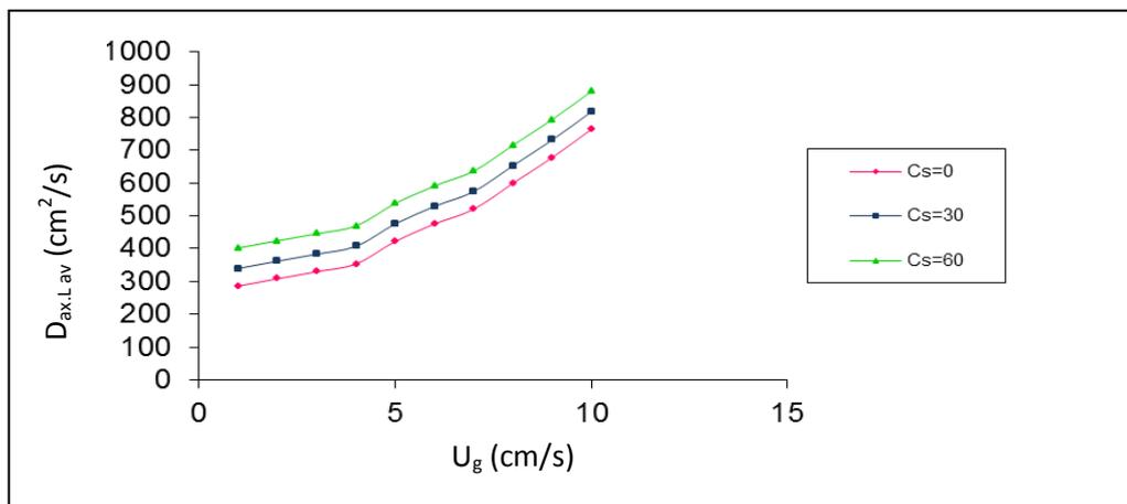
Fig.10. Effect of Superficial Gas Velocity and Solid Concentration on Average Axial Liquid Dispersion Coefficient at dp= 3mm.
