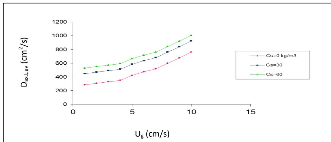
Fig. 12. Effect of Superficial Gas Velocity and Solid Concentration on Average Axial Liquid Dispersion Coefficient at dp= 0.7mm.
