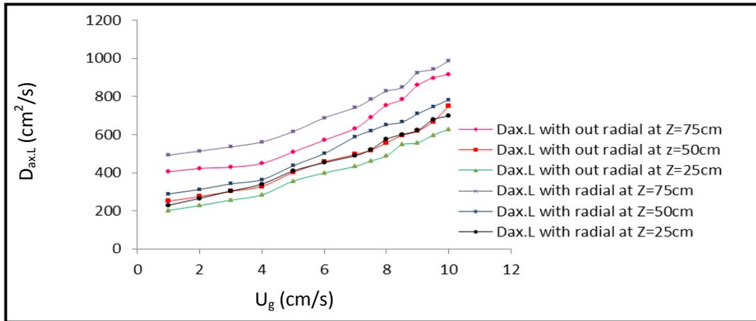
Fig. 3. Effect of Superficial Gas Velocity on Axial Liquid Dispersion Coefficient at Different Z and  $C_S=0$ .
