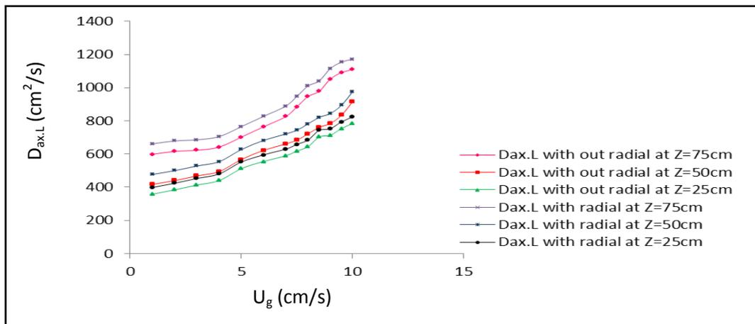
Fig. 7. Effect of Superficial Gas Velocity no Axial Liquid Dispersion Coefficient at Different Z, CS=60 and dp= 1.5mm.
