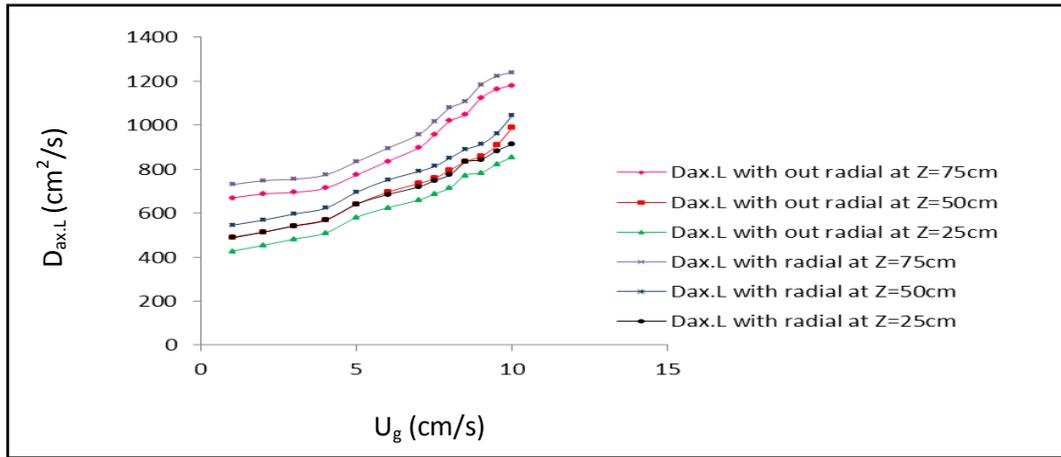
Fig. 9. Effect of Superficial Gas Velocity no Axial Liquid Dispersion Coefficient at Different Z, CS=60 and dp= 0.7mm
