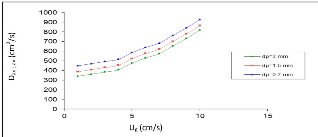
Fig. 13. Effect of Superficial Gas Velocity and Solid Concentration on Average Axial Liquid Dispersion Coefficient at CS= 30kg/m3.
