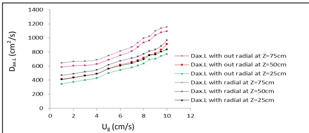
Fig. 8. Effect of Superficial Gas Velocity no Axial Liquid Dispersion Coefficient at Different Z, CS=30 and dp= 0.7mm.
