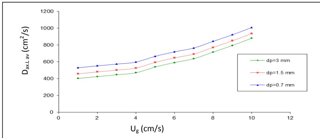
Fig. 14. Effect of Superficial Gas Velocity and Solid Diameter on Average Axial Liquid Dispersion Coefficient at CS= 60kg/m3
