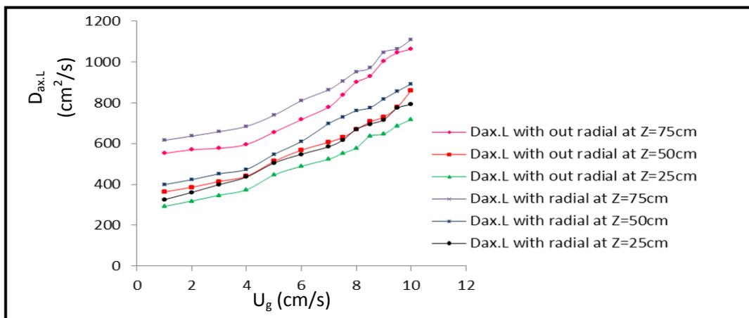
Fig. 5. Effect of Superficial Gas Velocity on Axial Liquid Dispersion Coefficient at Different Z,  $C_S=60$  and  $dp=3mm$ .
