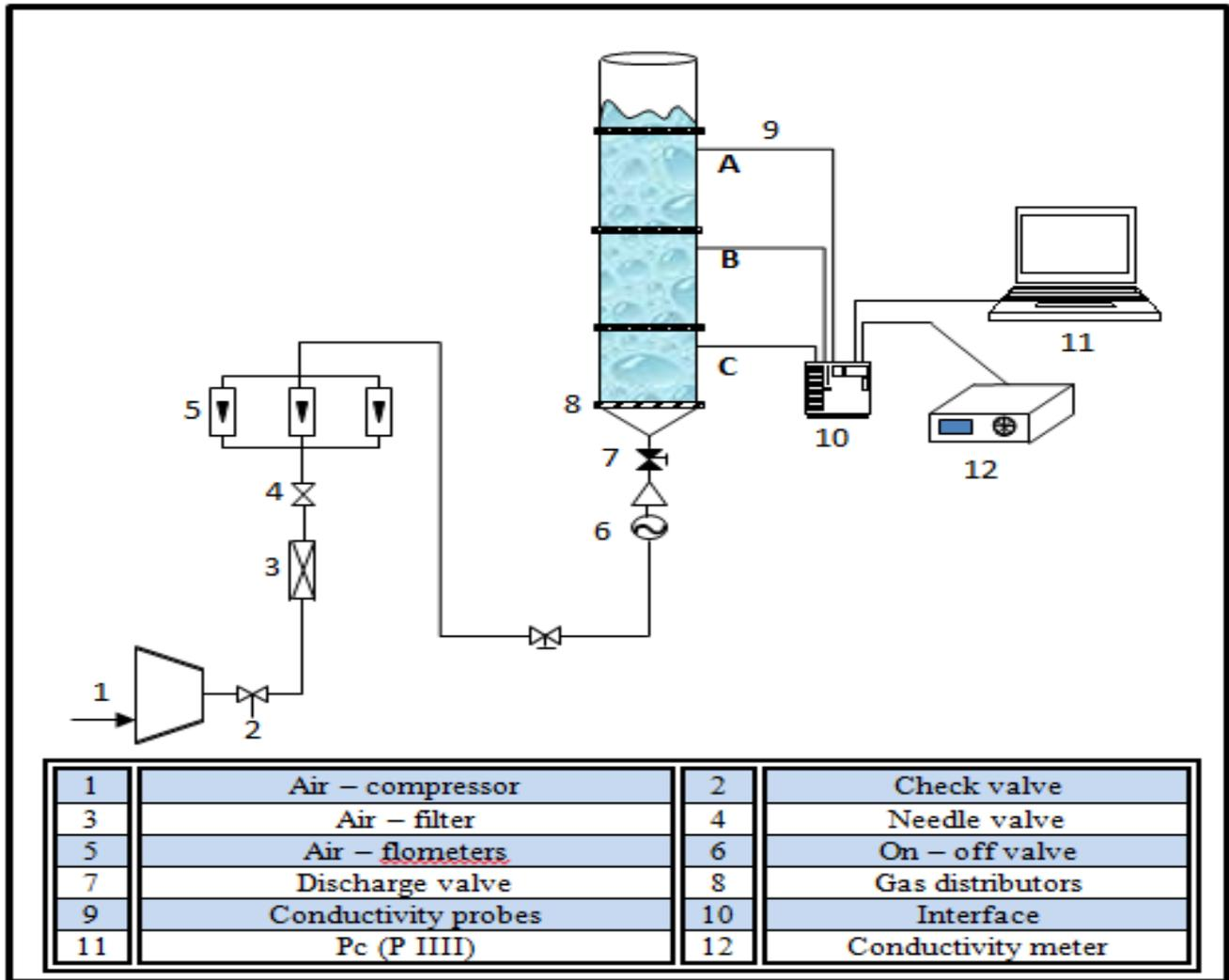
Fig.1. Schematic Diagram of the Experimental Apparatus.
