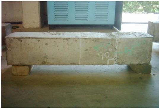
Plate (5) Beam with Vertical Construction Joint at Third Point without Stirrups after Testing .
