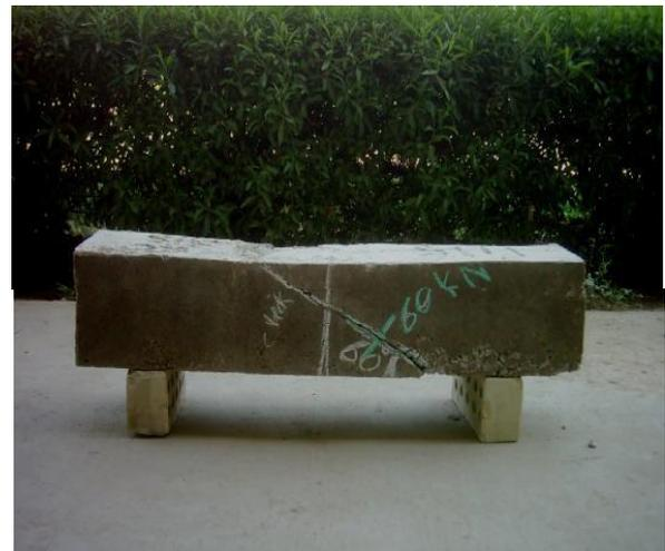
**Plate(4) Beam With  $60^\circ$  Inclined Construction Joint at Midspan After Testing.**
