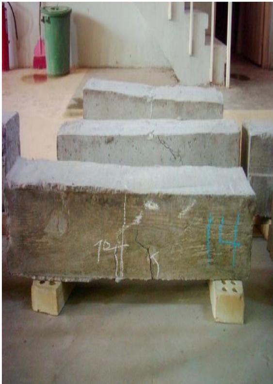
**Plate (3) Beam without Construction Joint (Reference Beam) After Testing .**
