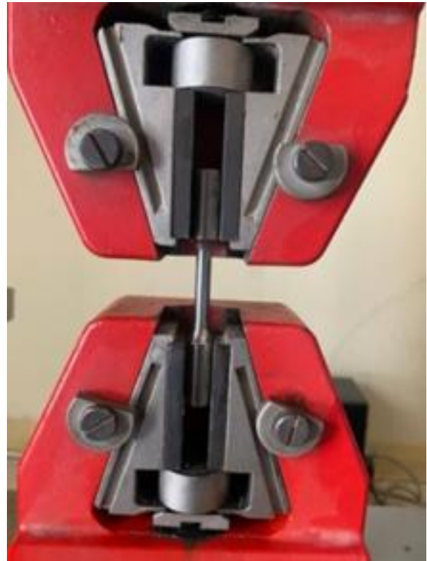
Fig. 2. Test machine holds the specimen under tension.
