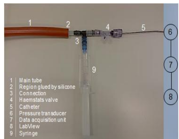
Fig. 2. Experimental setup applied, estimating compliance testing-based-pulse wave speed for the selected synthetic flexible tube, indicating all parts.
