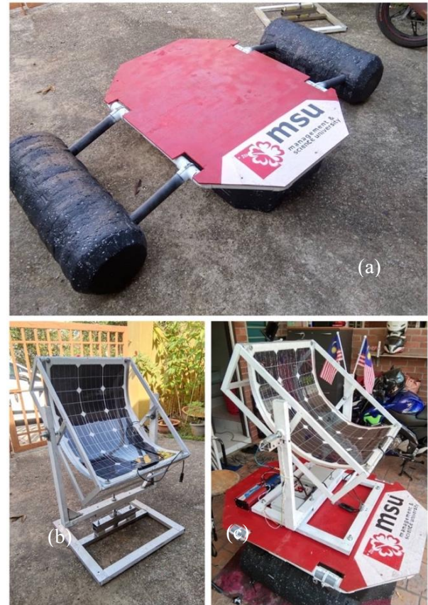
Fig. 9. (a) Floating pontoon, (b) curved trough collector and (c) single-axis tracking system.
