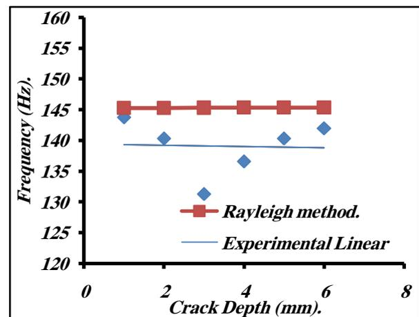
Fig. 11. The Comparison between the Experimental and Rayleigh Method Results at Different Crack Depths When the Crack lies at (42 cm) .
