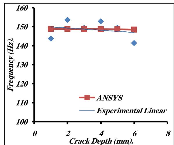
Fig. 5. The Comparison between the Experimental and ANSYS Results at Different Crack Depths When the Crack lies at (22 cm) .
