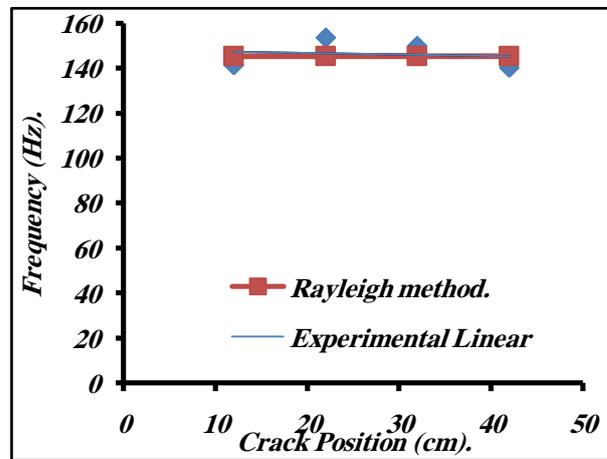
Fig. 17. The Comparison between the Experimental and Rayleigh Method Results at Different Crack Position When the Crack Depth is (2mm) .
