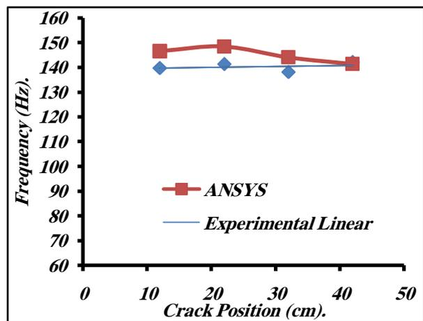
Fig. 16. The Comparison between the Experimental and ANSYS Results Different at Crack Position When the Crack Depth is (10mm) .
