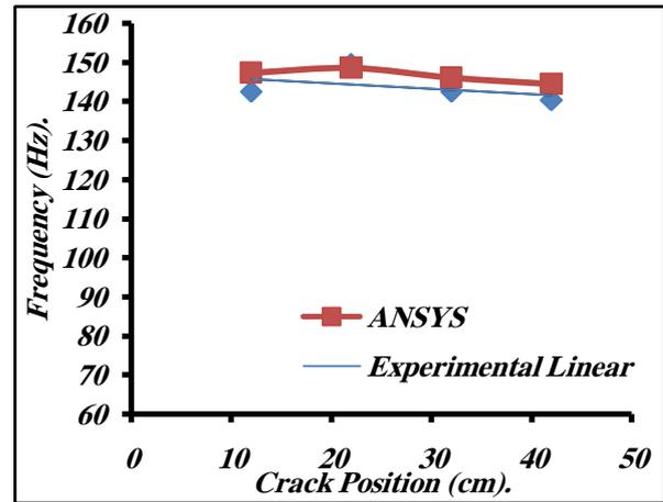
Fig. 15. The Comparison between the Experimental and ANSYS Results at Different Crack Position When the Crack Depth is (8mm).
