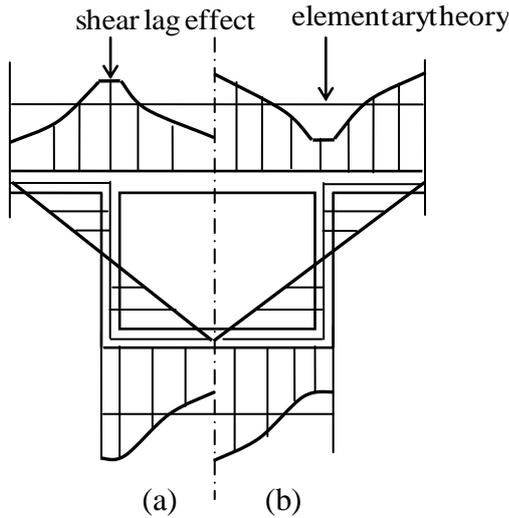
Fig. 2. Shear Lag Effect (a) Positive shear lag, b) Negative Shear lag (Chang and Zhang, 1987).
