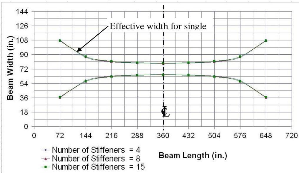
Fig. 10. Effect of Distribution of Stiffeners on the Distribution of the Effective Flange Widths.
