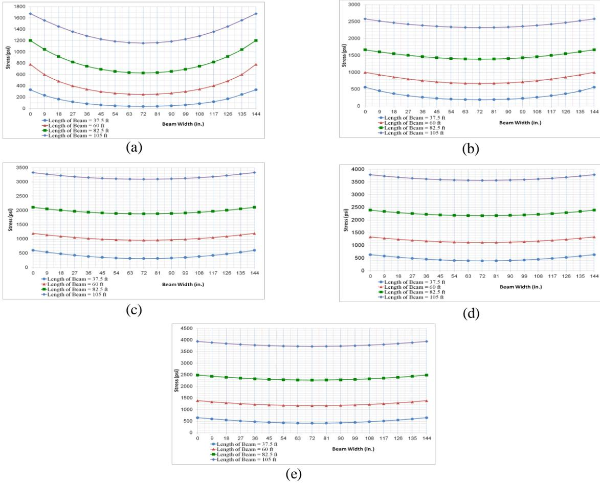
Fig. 15. Effect of Length of Girder on Top Flange Stress Distribution.
