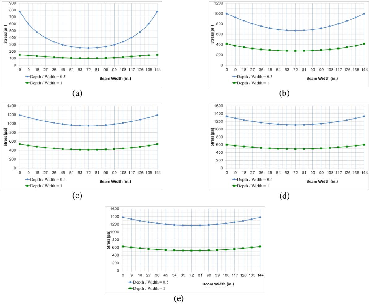
**Fig. 13. Effect of Depth/Width on Top Flange Stress Distribution.**
