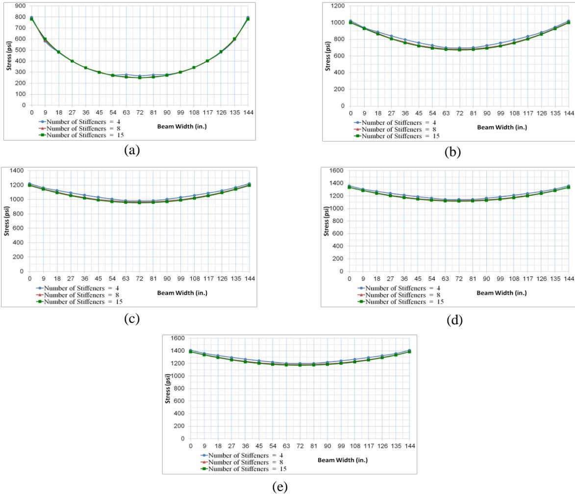
Fig. 9. Effect of Distribution of Stiffeners on Top Flange Stress Distribution .
