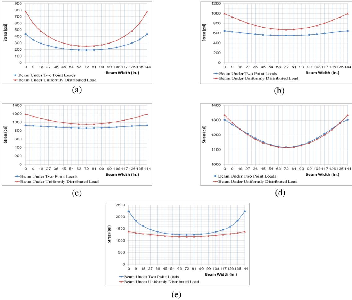
**Fig. 11. Effect of Loading on Top Flange Stress Distribution.**
