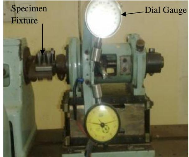
Fig. 2-6. a) AVERY Fatigue Testing Machine Type 7305, b) Close up of Specimen Fixture.
