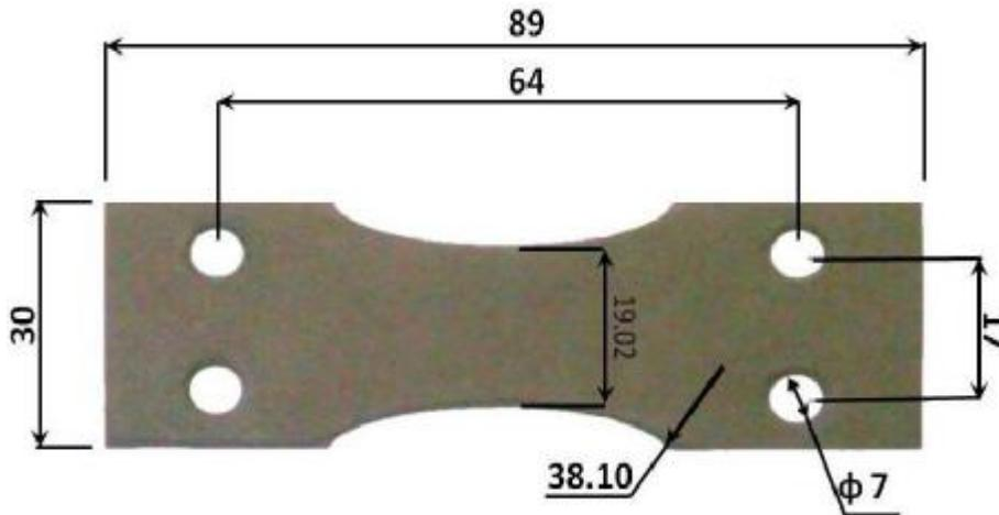
Fig. 2-5. Fatigue Specimens (all Dimension in mm) [12].
