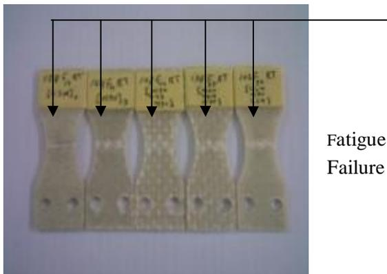
Fig. 2-7. Fatigue Failure of Composite Specimens.
