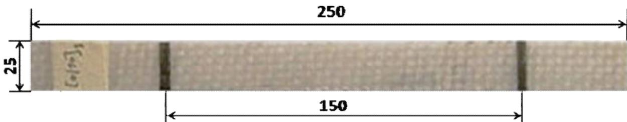
**Fig. 2-2. Composite Tensile Test Specimen (Dimensions in mm).**
