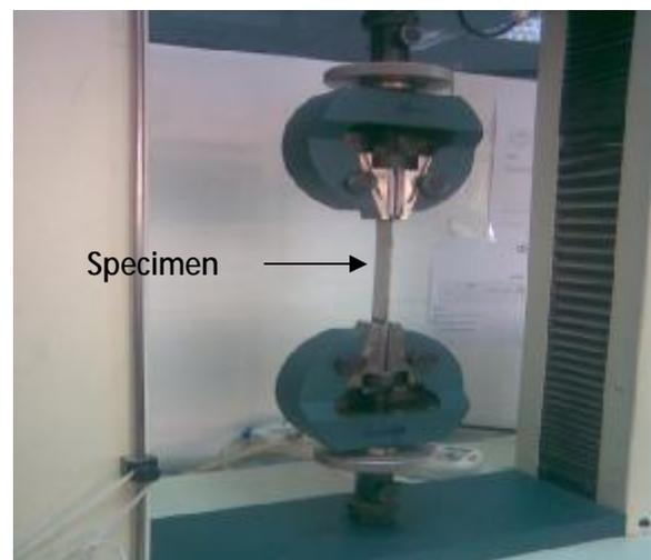
**Fig. 2-3. Close Up of Specimen Fixture.**
