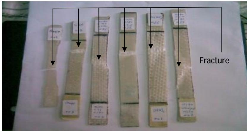
Fig. 2-4. Examples of Tensile Specimens after Failures.
