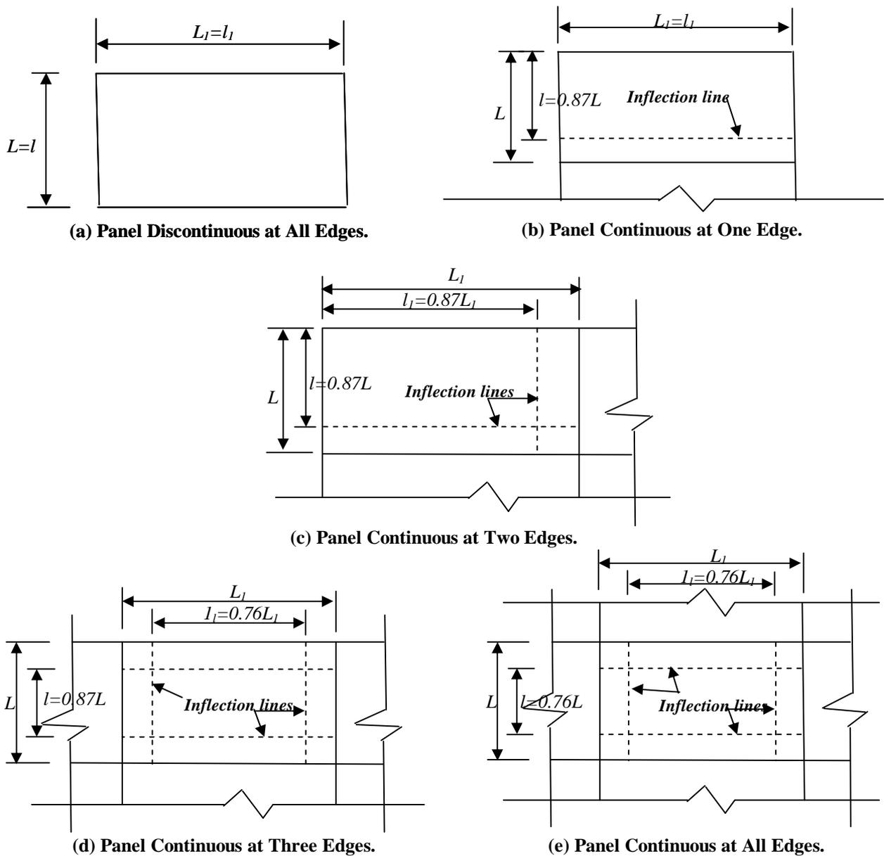
Fig. 2. Inflexion Lines in Reinforced Concrete Panels According to ACI 63 Code.
