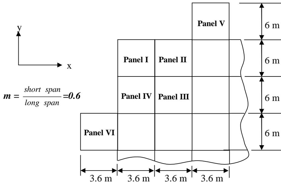
Fig. 3. Proposed Panels of m=0.6 Used for the Comparison between the Proposed Method and Other Methods.
