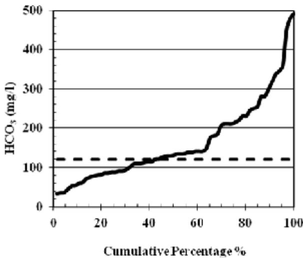
Fig. 9.  $\text{HCO}_3$  Values vs. Cumulative Percentage of Samples.
