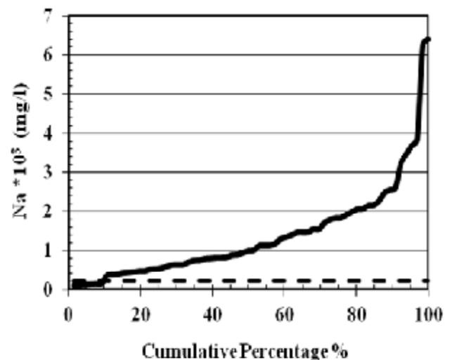
Fig. 5. Na Values vs. Cumulative Percentage of Samples.
