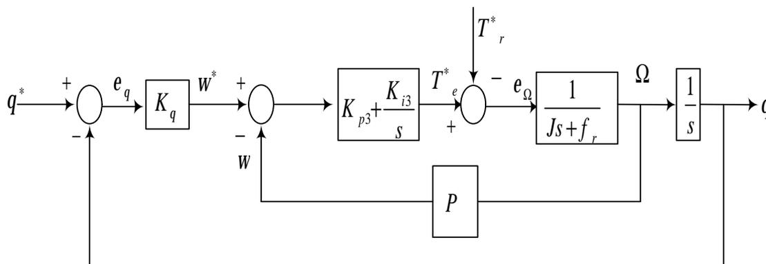
Fig. 1. Block Diagram of Position Regulation.
