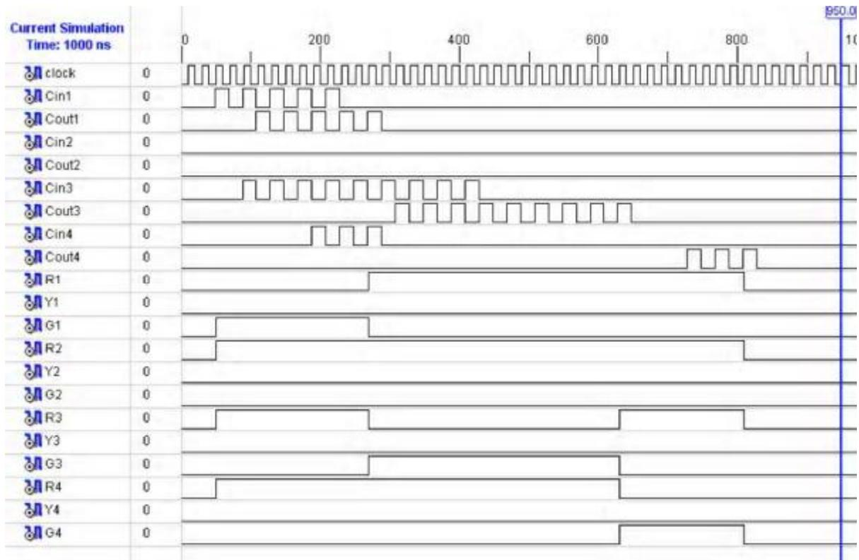
Fig.6. Simulation Behavioral Model when One Side had Completed Passage of all Vehicles and the others have Vehicles.
