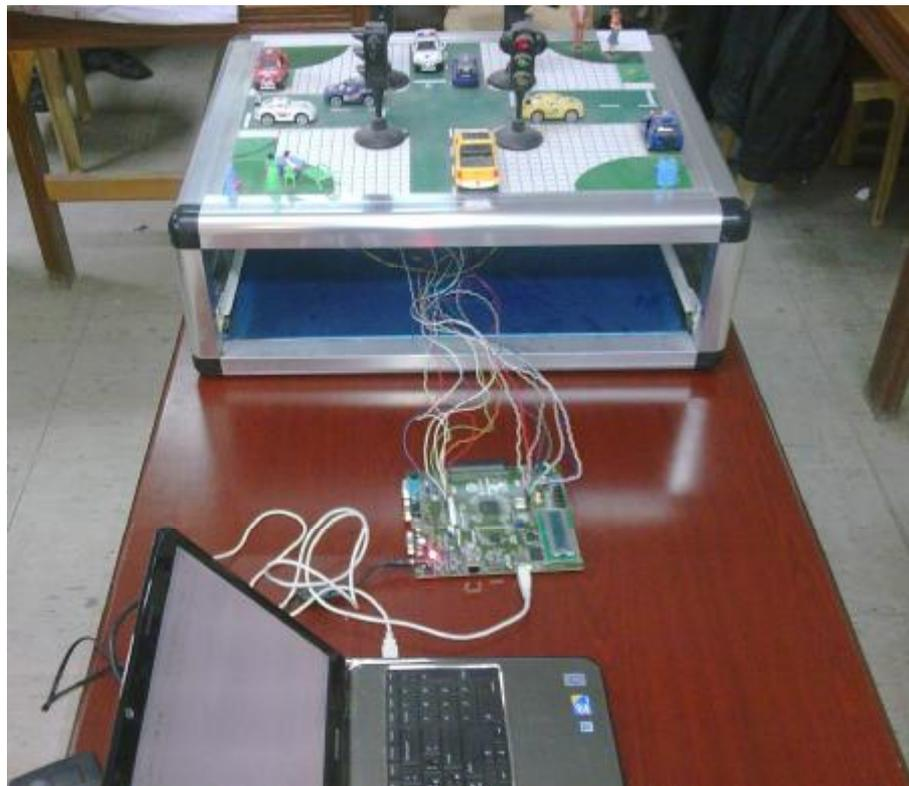
Fig.9. The Proposed Model Implementation Using the Spartan-3A XC3S700A FPGA kit.
