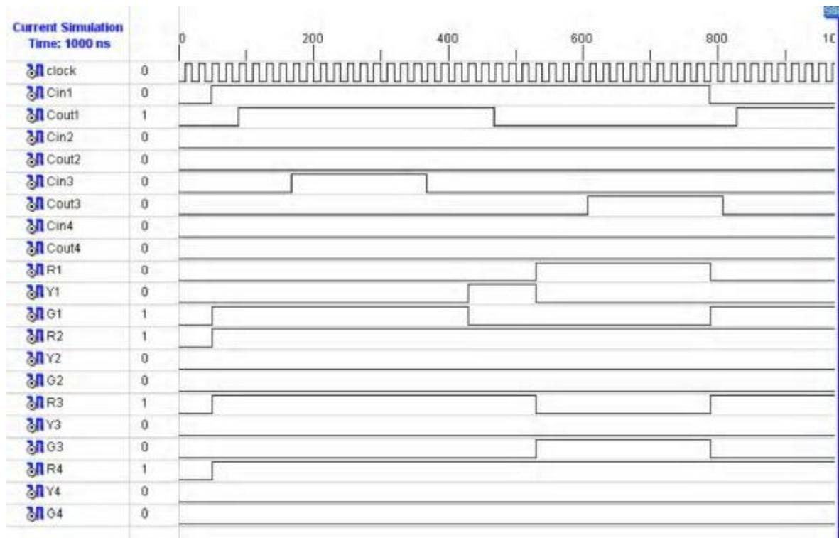
Fig. 8. Simulation Behavioral Model When One Side Is Full And Exceeds The Time Desired.
