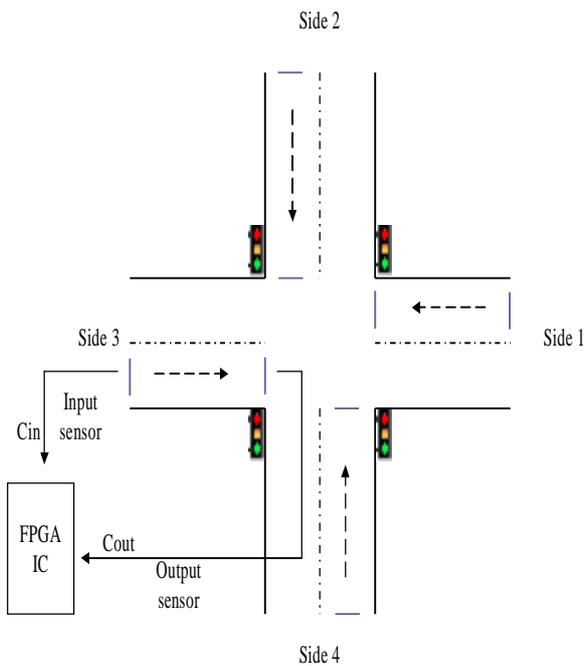
**Fig. 1. Mechanism of Sensors on Both Ends of Each Side of the Intersection.**
