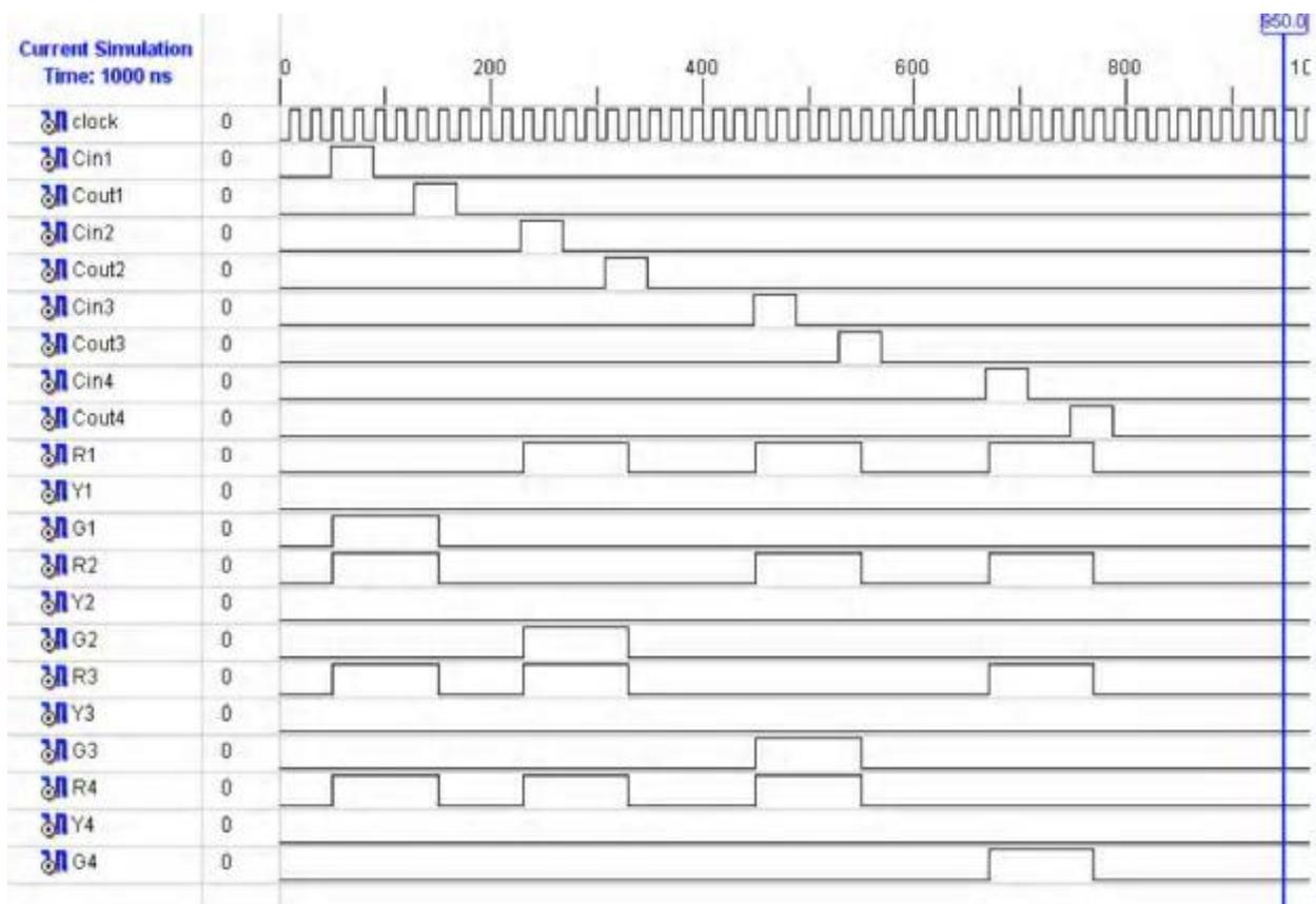
Fig. 5. Simulation Behavioral Model when One Side has Vehicles and others are Empty.
