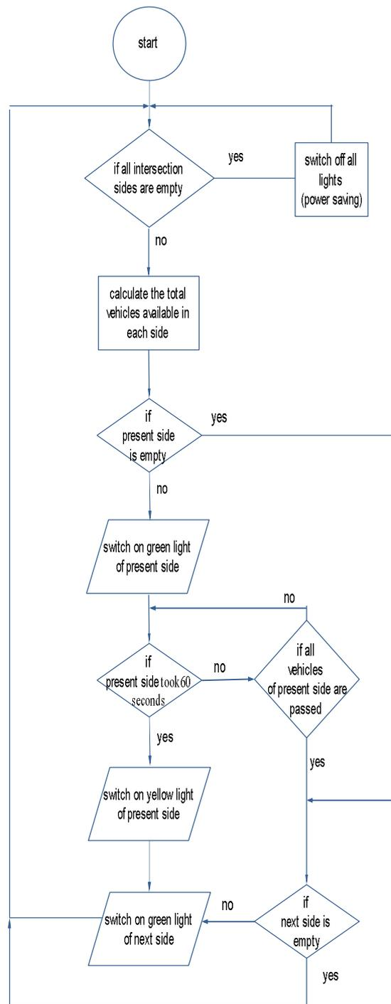
**Fig. 2. The Flowchart of the Proposed Traffic Light.**
