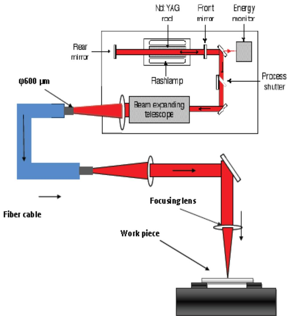
Fig. 3. Experimental Setup for Nd-YAG JK760TR.
