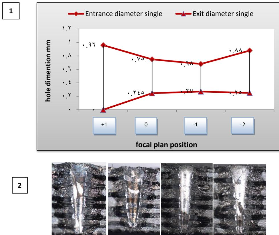
Fig. 6. (1) Effect of fpp on the Dimensions of Laser Drilled Microholes ( $f = 10$  Hz), (2) Optical Picture Showing Changing Crater Dimensions for Different Fpp.
