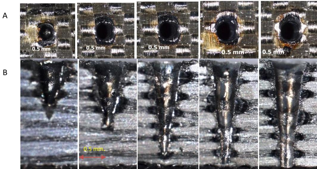
**Fig. 9. A- Optical Images of the Cross-Section of FR-4 Drilled Hole at 2 ms Pulse Width. B- Effect of Peak Power at 2ms Pulse Width on the Hole Dimension.**
