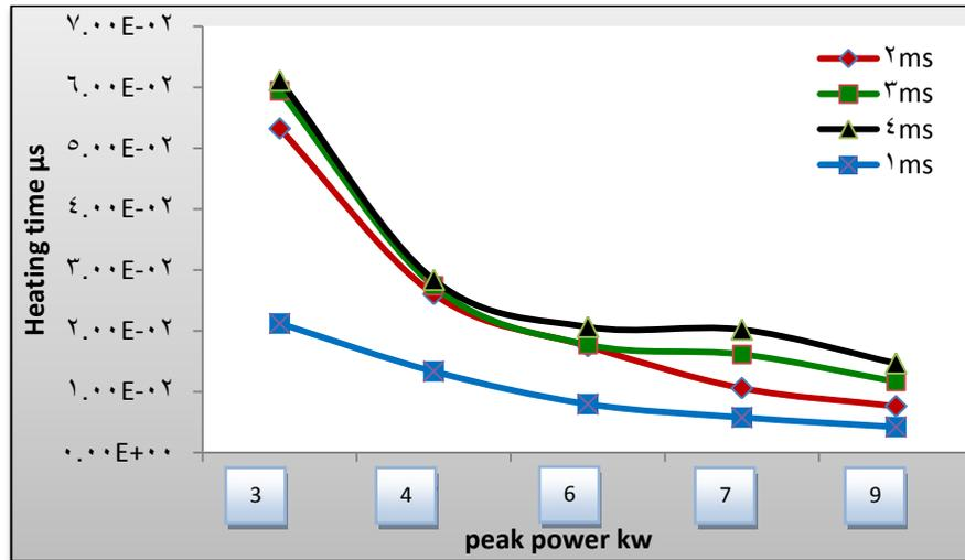
Fig. 7. Effect of Laser Power on the Heating Stage.
