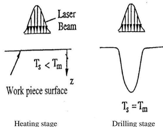
**Fig. 1. Heating and Material Removal Stages of Laser Drilling [9].**
