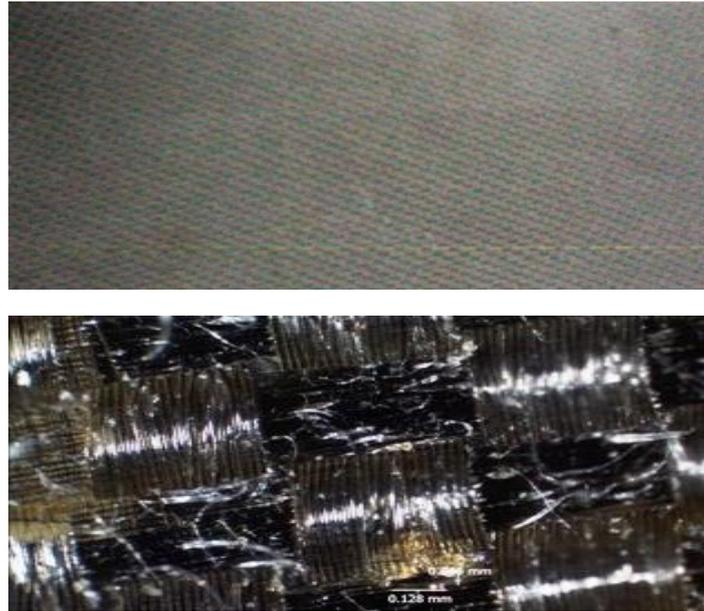
Fig. 5. A: 2116 Glass Fiber Composite FR-4 Work Piece: B: High Magnification (16x) Showing Glass Fiber.
