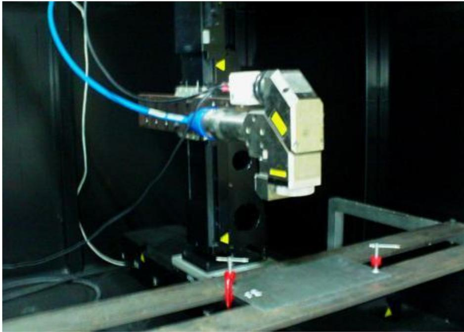
**Fig. 4. Millisecond Pulsed Nd:YAG Laser Head.**
