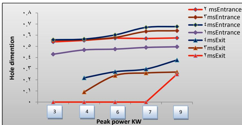
Fig. 8. Effect of Laser (Peak Power, Pulse Duration) on the Dimensions of Laser Drilled Micro Holes in FR-4, ( f = 10 Hz , and fpp = -1).
