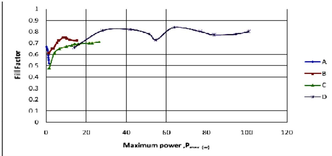
Fig. 8. Variation of Solar Cell Fill Factor with Maximum Power for the Four Solar Cell Types.
