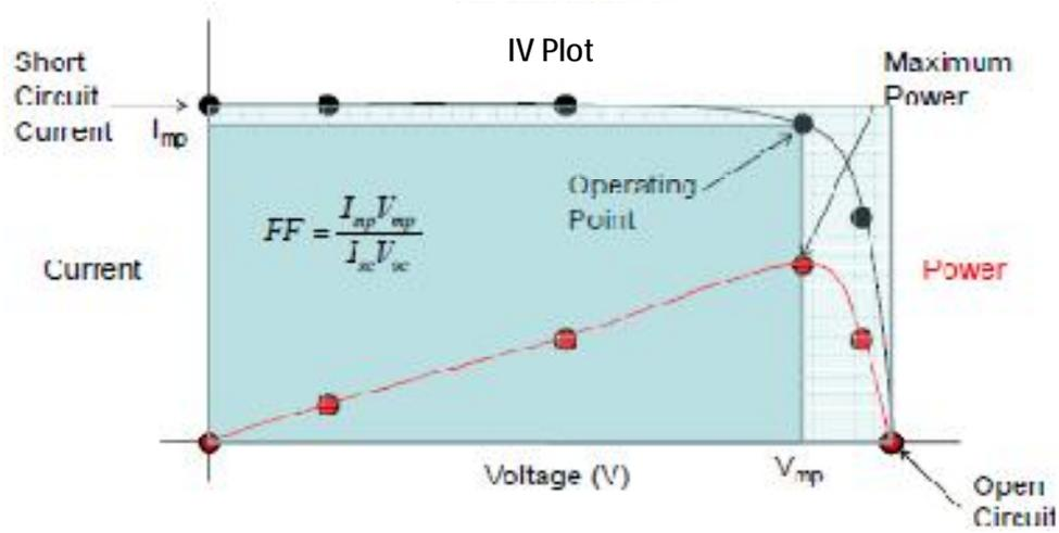
Fig .2. Square Area is The Maximum Power Output of the Solar Cell.
