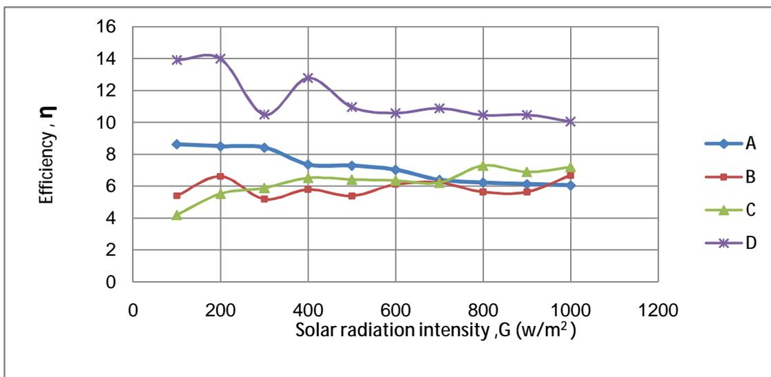
Fig. 7. Variation of Solar Cell Efficiency with Solar Radiation Intensity for the Four Solar Cell Types.
