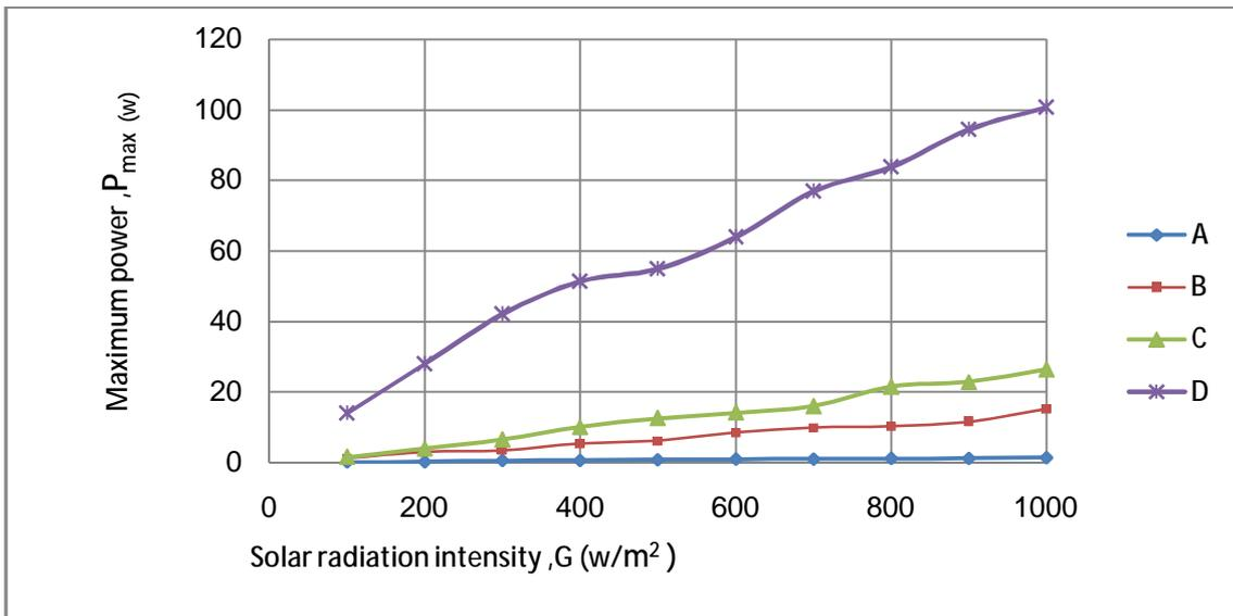
Fig. 6. Variation of Solar Cell Maximum Power with Solar Radiation Intensity for the Four Solar Cell Types.
