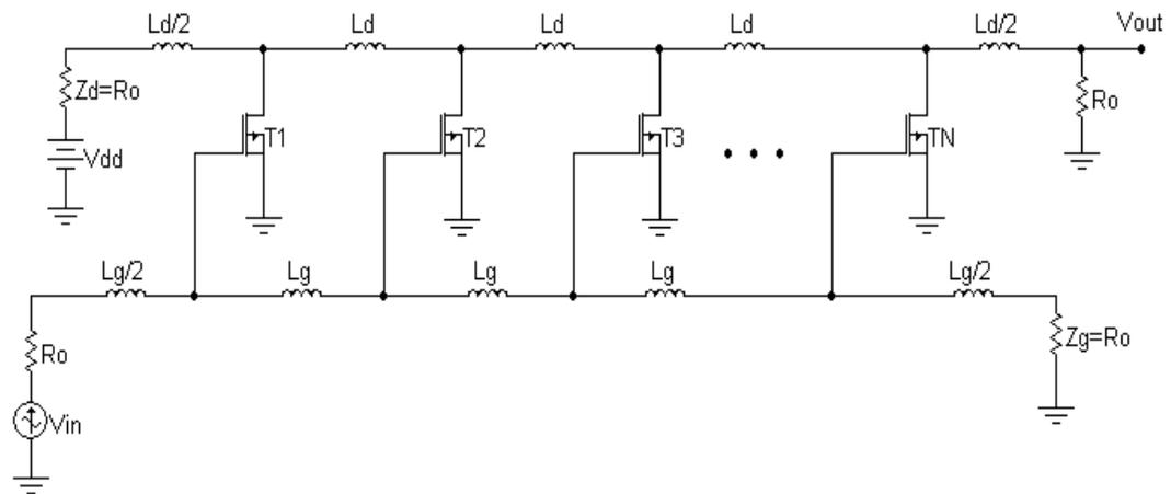
Figure(1) Schematic circuit of N-stages CDA
