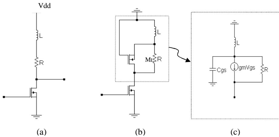
Figure(4) Single stage of DA.(a)simple common source amplifier.(b)the amplifier with active inductor.(c)the equivalent model of the active inductor.
