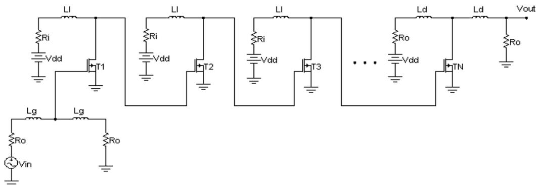
Figure(2) Schematic circuit of N-stages CSSDA
