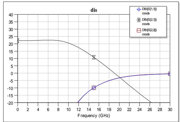
Figure(7) Simulated S-parameters in the CSSDA with active inductors ( $L_1= 0.1$  nH)
