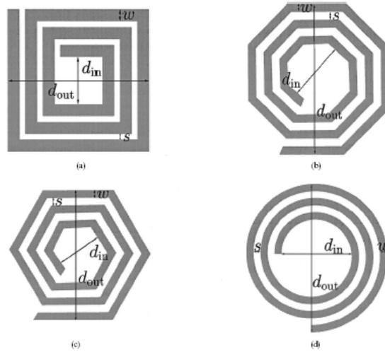
Figure(3) On-chip spiral inductor realizations: (a) square, (b) hexagonal, (c) octagonal, and (d) circular.
