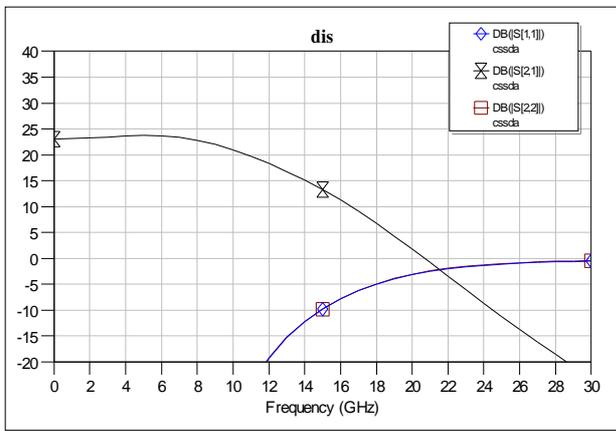
Figure(6) Simulated S-parameters in the CSSDA with passive inductors ( $L_1= 0.42$  nH)
