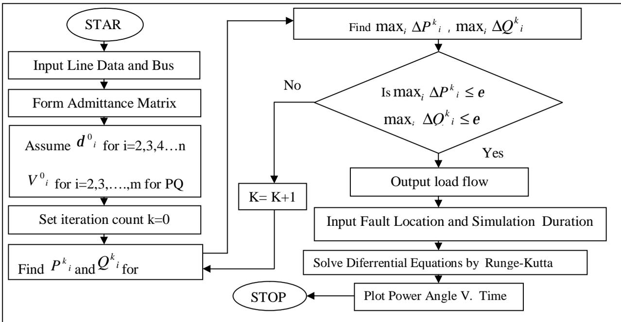
Fig. 3.The Flow Chart of the Transient Stability Program.
