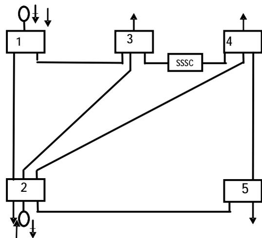
Fig. 4. Single Line Diagram of IEEE-5 Bus Network with SSSC.
