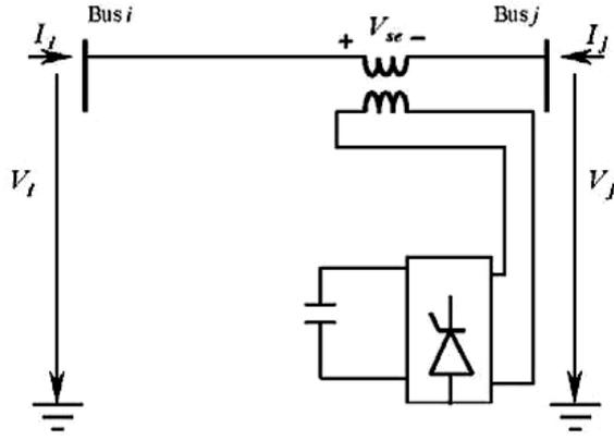
Fig. 1. The Operating Principles of SSSC.
