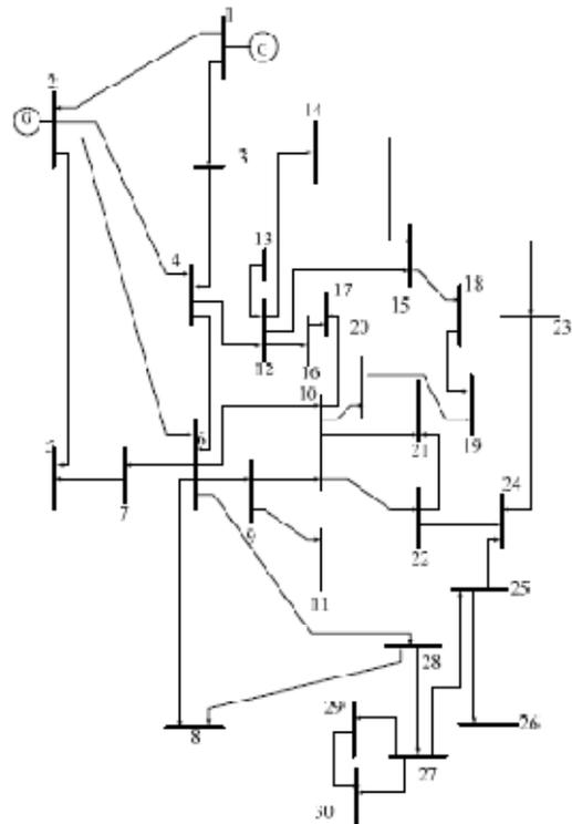
Fig. 8. Single Line Diagram of IEEE-30 Bus System.
