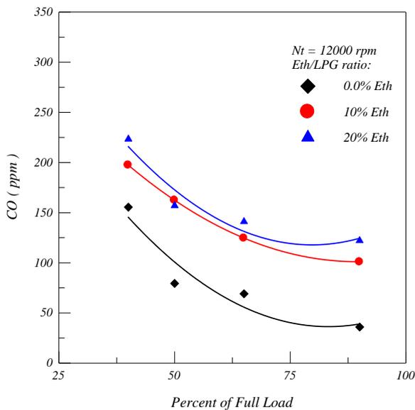
Fig. 6. Effect of Engine Loading on CO Emission.
