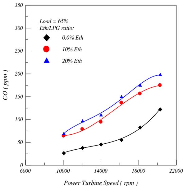
Fig. 3. Effect of Power Turbine Speed on CO Emission.
