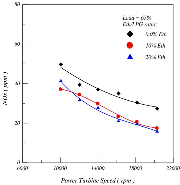
Fig. 2. Effect of Power Turbine Speed on No<sub>x</sub> Emission.
