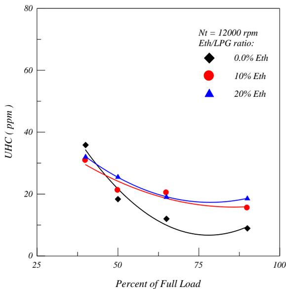
Fig. 7. Effect of Engine Loading on UHC Emission.
