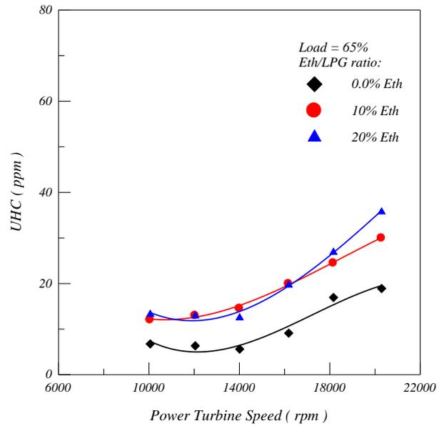
Fig. 4. Effect of Power Turbine Speed on UHC Emission.
