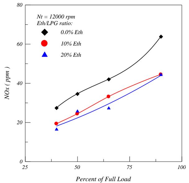
Fig. 5. Effect of Engine Loading on No<sub>x</sub> Emission.
