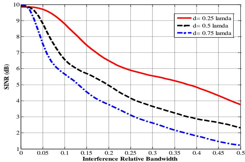
Fig. 5. SINR plot versus interference relative bandwidth for different interelements spacing
