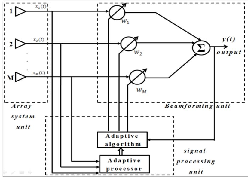
Fig. 1. M-elements adaptive array system.
