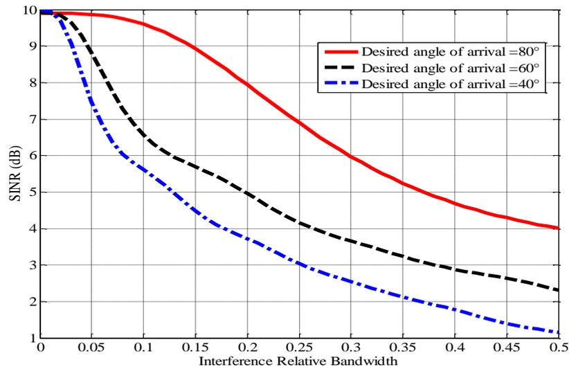
Fig. 3. Output SINR plot versus interference relative bandwidth for different desired signals angle of arrival.
