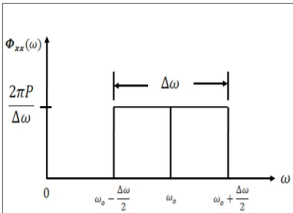
Fig. 2. The power spectral density of received signal.
