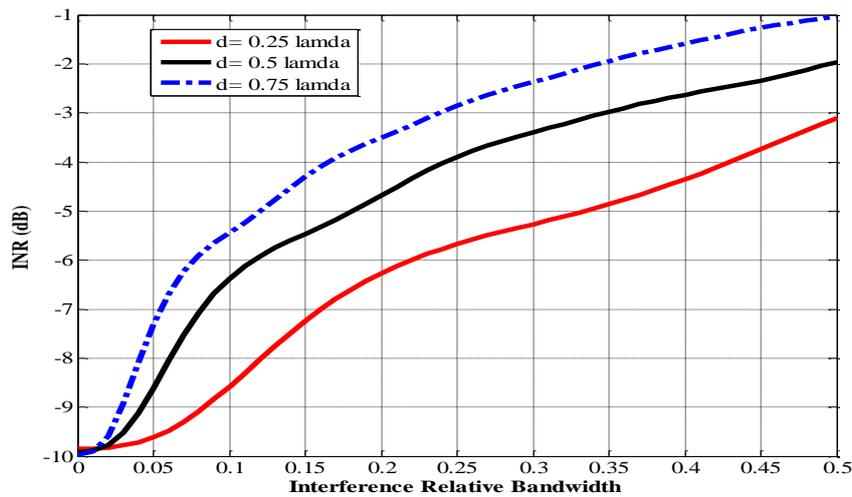
Fig. 6. INR plot versus interference relative bandwidth for different interelements spacing
