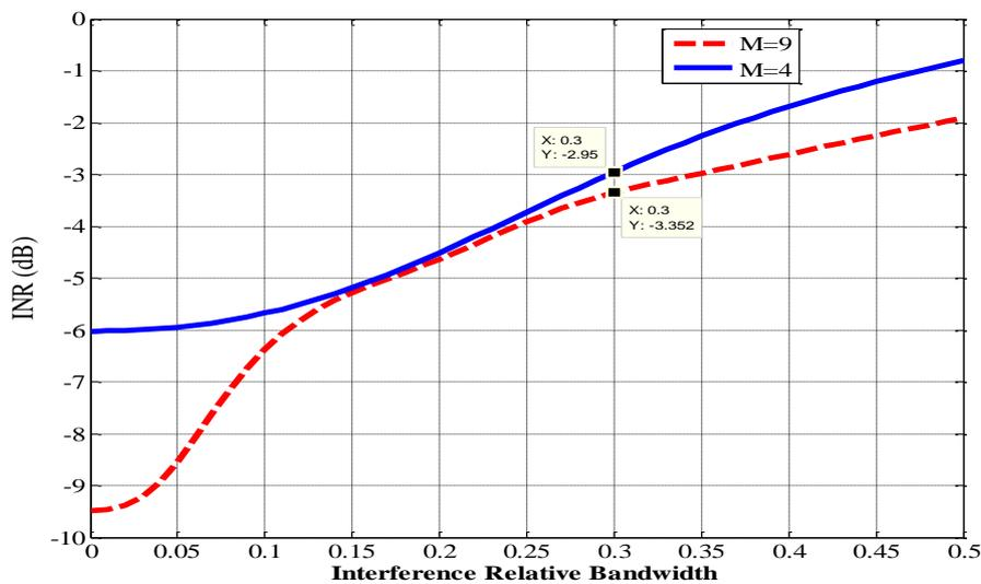
Fig. 8. INR plot versus interference relative bandwidth for different number of antennas.
