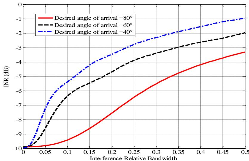
Fig. 4. Output INR plot versus interference relative bandwidth for different desired signals angle of arrival.
