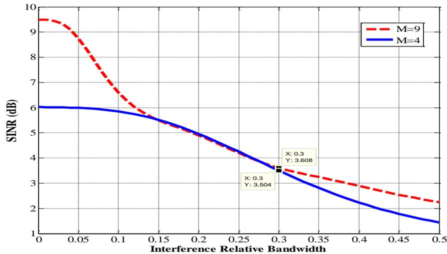
Fig. 7. SINR plot versus interference relative bandwidth for different number of antennas.
