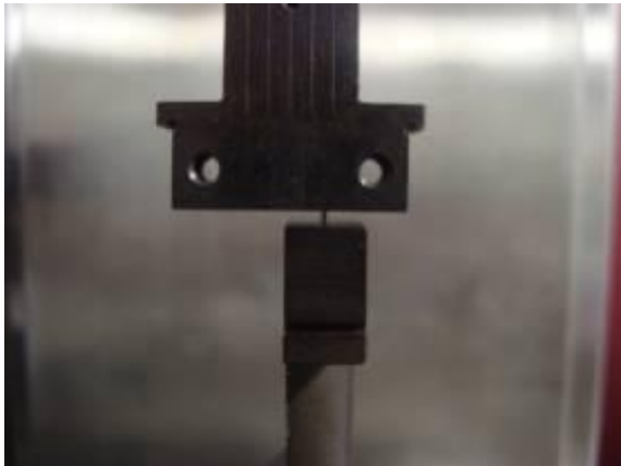
Fig.1. Ball compression fixture within Rheometric Solids Analyzer machine (Compliance 6.996E-05 mm/gm.)
