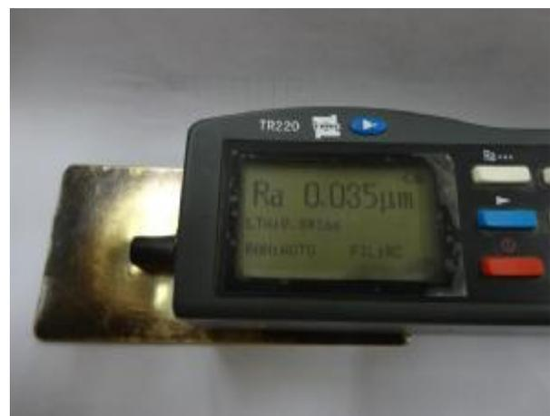
**Fig. 5. Surface roughness tester, (TR-220).**
