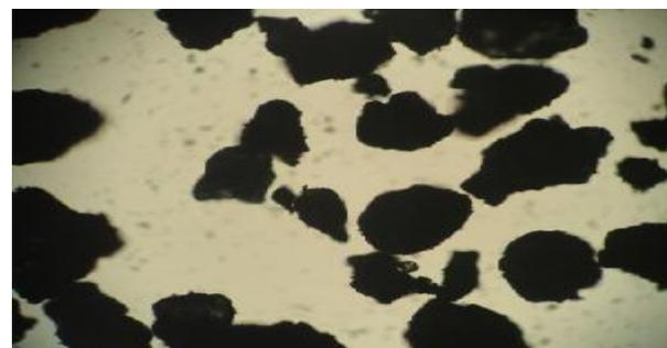
Fig. 3. SEM (X 100) of magnetic abrasive particles.
