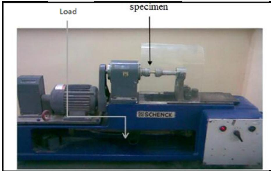
Fig. 2. PUNN rotary fatigue bending machine.
