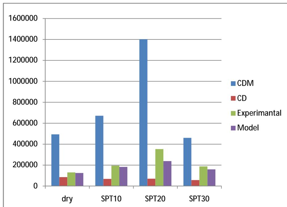
Fig. 4. shows the High-Low cumulative fatigue life prediction for four methods.
