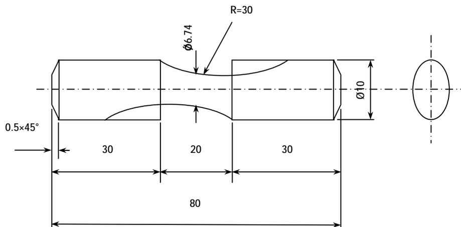
**Fig. 1. Specimen geometry and dimensions for fatigue test (all dimensions in mm).**
