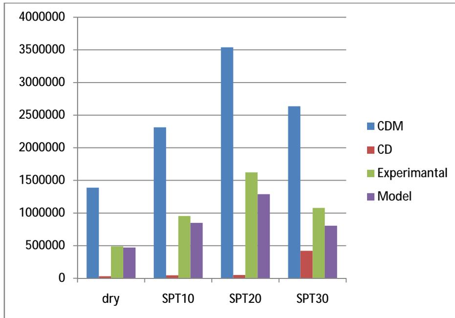
Fig. 3. shows the Low-High cumulative fatigue life prediction for four methods.
