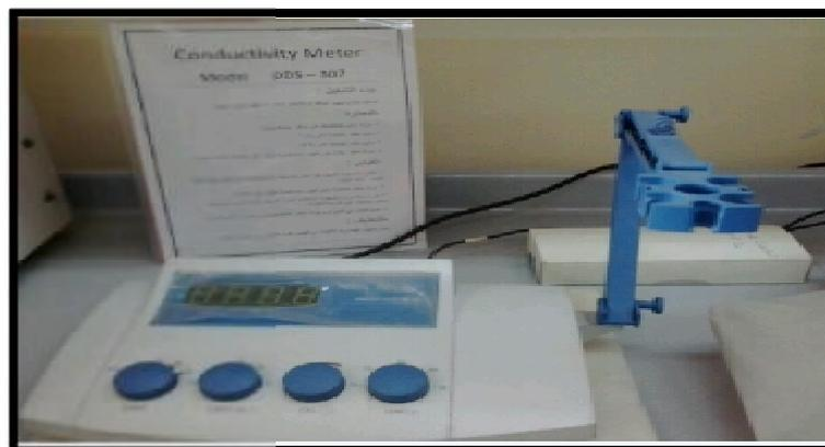
**Fig.3.** Digital electrical conductivity meter.
