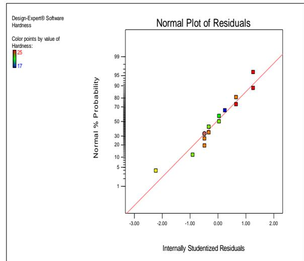
Fig. 6. Normal probability plot for hardness data.
