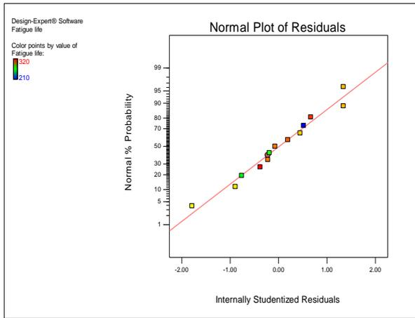
Fig. 1. Normal probability plot for fatigue life data.
