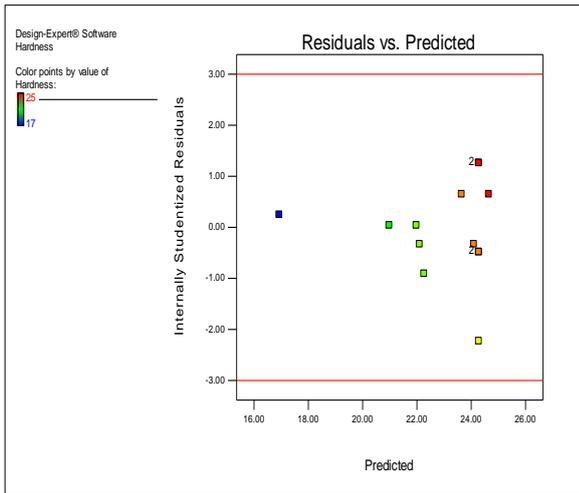
Fig. 7. Residual versus predicted responses for harness data.
