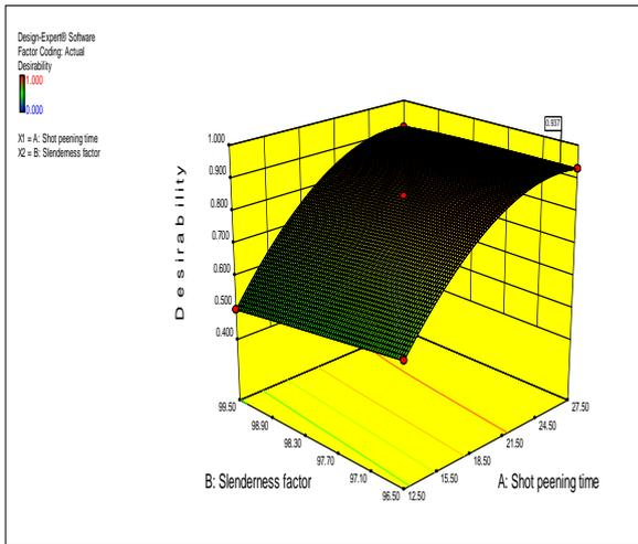
Fig. 13.3D surface plot for desirability as a function of shot peening time and slenderness ratio.
