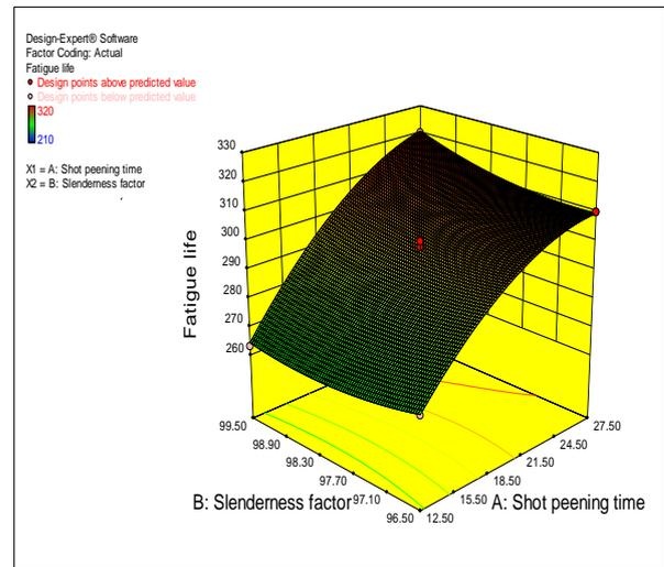
Fig. 5. 3D graph of fatigue life as a function of shot peening time (min) and slenderness ratio.
