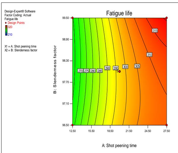
Fig. 3. Contour graph of fatigue life as a function of shot peening time (min) and slenderness ratio.
