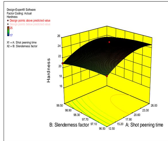
Fig. 10. 3D graph of hardness (HRC) as a function of shot peening time (min) and slenderness ratio.
