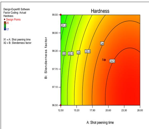
Fig. 8. Contour graph of hardness (HRC) as a function of shot peening time and slenderness ratio.
