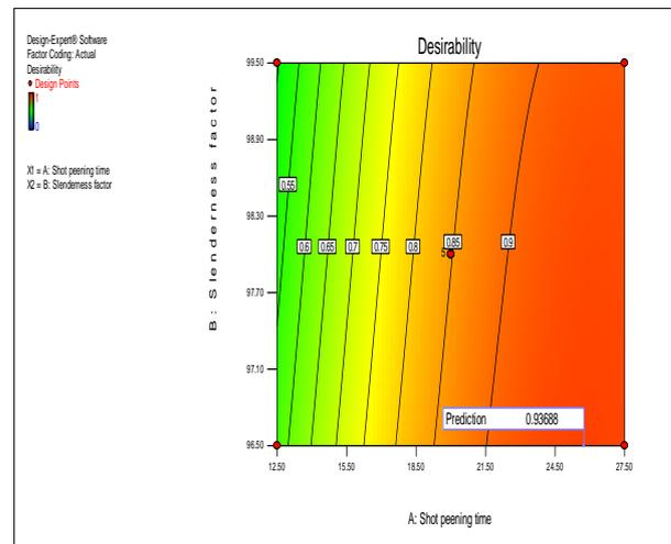
Fig. 12. 2D contour for desirability as a function of shot peening and slenderness ratio.
