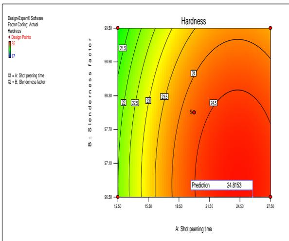
Fig. 15. The optimum value of hardness (HRC).
