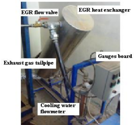
Fig. 2. EGR assembly used in the present study.
