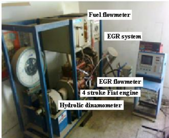
Fig. 1. Photographic picture for the experimental rig.
