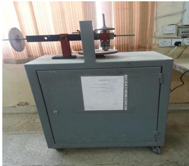
**Fig.1. Pin on disc wear apparatus.**
