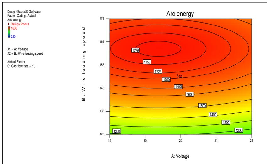
**Fig. 16. Contour Graph of Arc Energy as A Function of Voltage and Wire Feeding Speed at Gas Flow Rate 8 L/min.**
