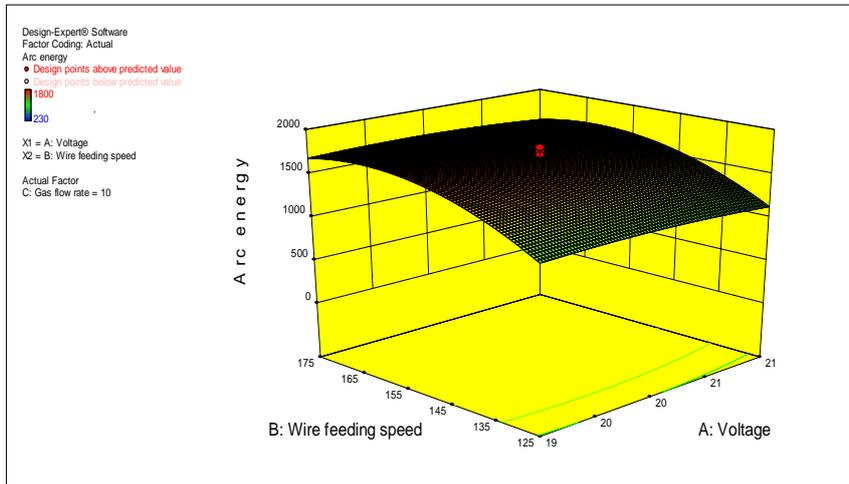
Fig. 18. 3D Graph of Arc Energy as A function of Voltage and Wire Feeding Speed at Gas Flow Rate 10 L/min.
