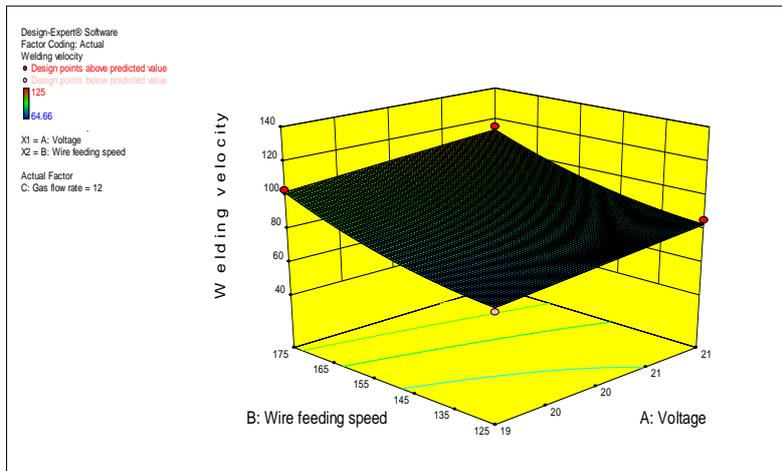
Fig. 10. 3D Graph of Welding Velocity As a function of Voltage and Wire Feeding Speed at Gas Flow Rate 12 L/min.
