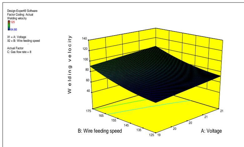
Fig. 8. 3D Graph of Welding Velocity as A function of Voltage and Wire Feeding Speed at Gas Flow Rate 8 L/min.
