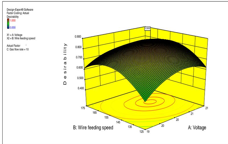
Fig. 21. 3D Graph for Desirability as A function Of Voltage and Wire Feeding Speed at Gas Flow Rate 10 L/min.
