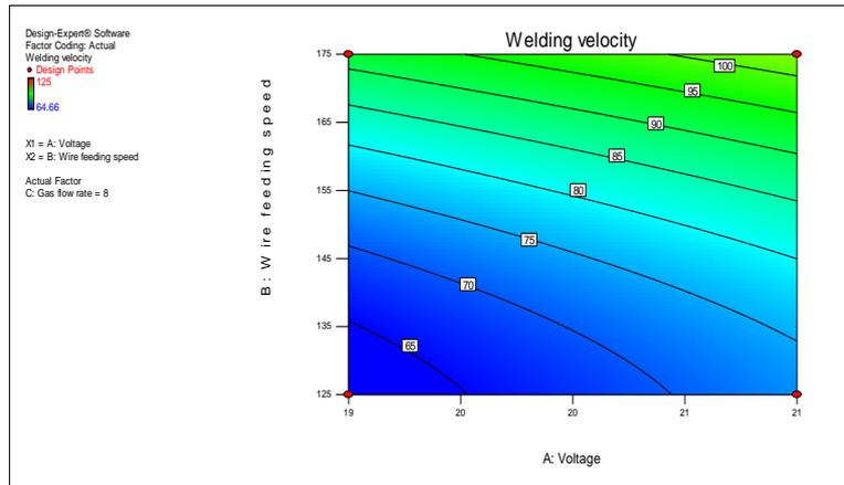
Fig. 6. Contour Graph of Welding Velocity as function of Voltage and Wire Feeding Speed Gas Flow Rate 10 L/min.
