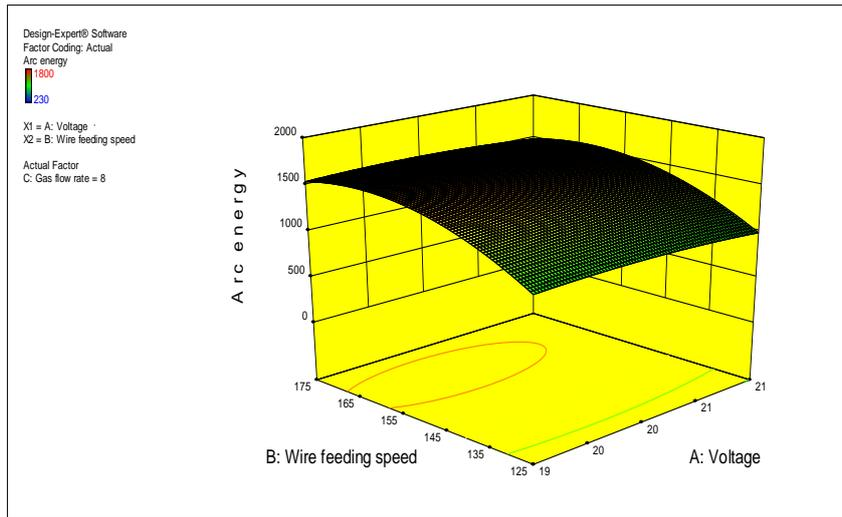
Fig. 17. 3D Graph of Arc Energy as A function of Voltage and Wire Feeding Speed at Speed at Gas Flow Rate 10 L/min.
