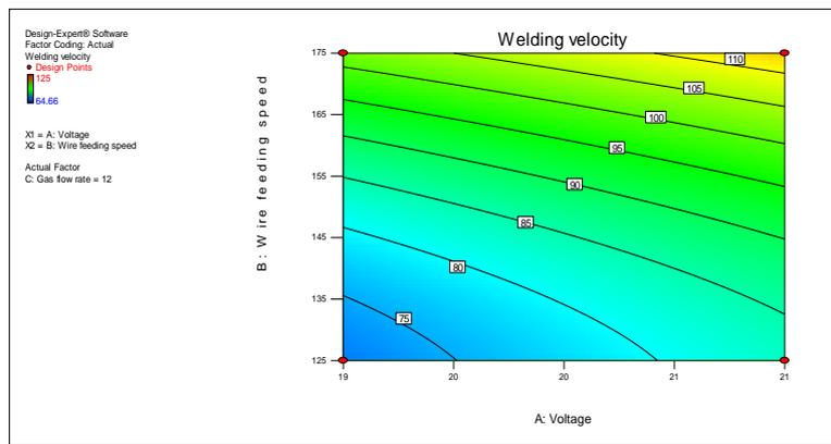
Fig. 7. Contour Graph of Welding Velocity as A function of Voltage and Wire Feeding Speed Gas Flow Rate 12 L/min.
