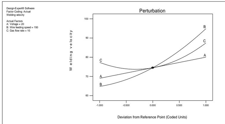
Fig. 4. Perturbation of Welding Velocity on Wire Feeding Speed and Gas Flow Rate.
