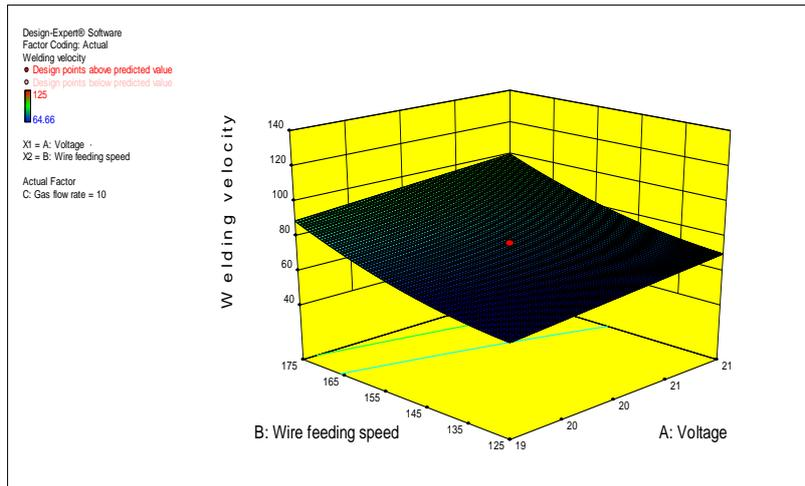
Fig. 9. 3D Graph of Welding Velocity as A function of Voltage and Wire Feeding Speed at Gas Flow Rate 10 L/min.
