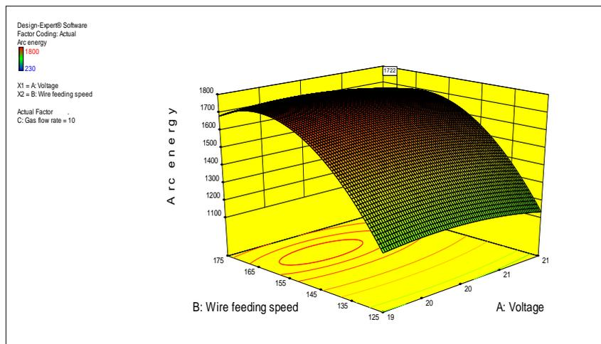
Fig. 23. The Optimum Value for Arc Energy At 10L/min Gas Flow Rate.
