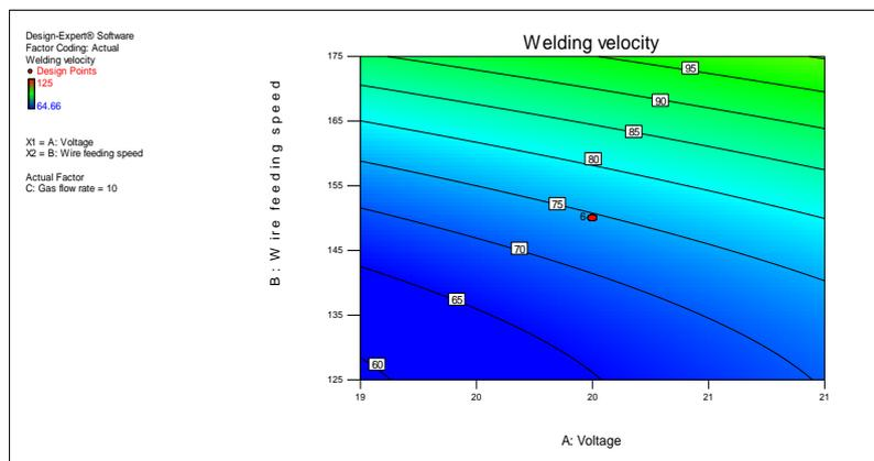
Fig. 5. Contour Graph of Welding Velocity as A function of Voltage and Wire Feeding Speed Gas Flow Rate 8 L/min.
