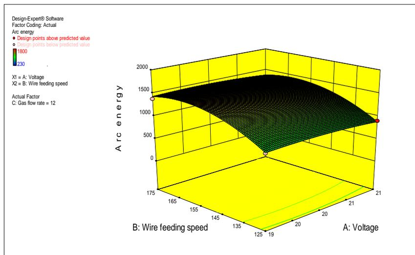
Fig. 19. 3D Graph of Arc Energy as A function of Voltage and Wire Feeding Speed at Gas Flow Rate 12 L/min.
