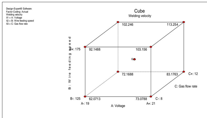
Fig. 11. Cube Shape of Welding Velocity.
