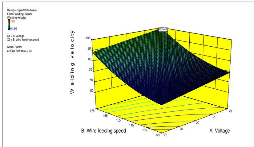
Fig. 22. The Optimum Value for Welding velocity at 10 L/min Gas Flow Rate.
