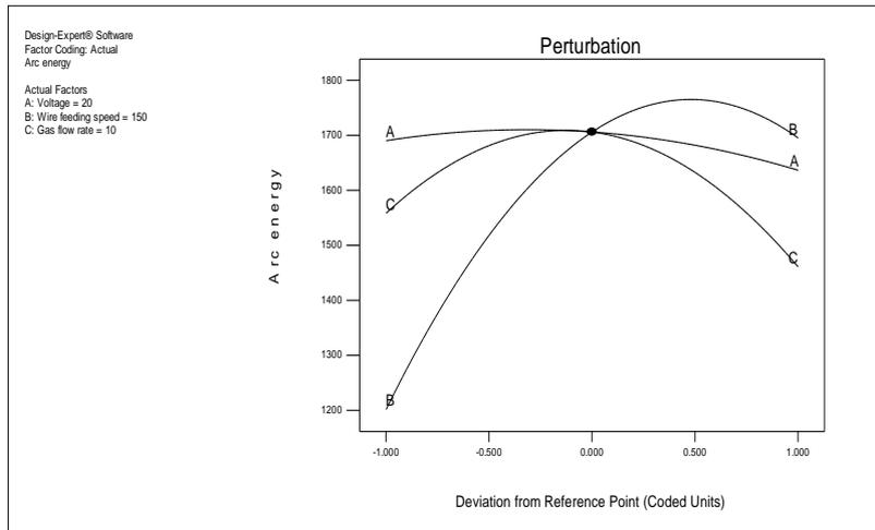
**Fig. 15. Perturbation of Arc Energy on Wire Feeding Speed and Gas Flow Rate.**
