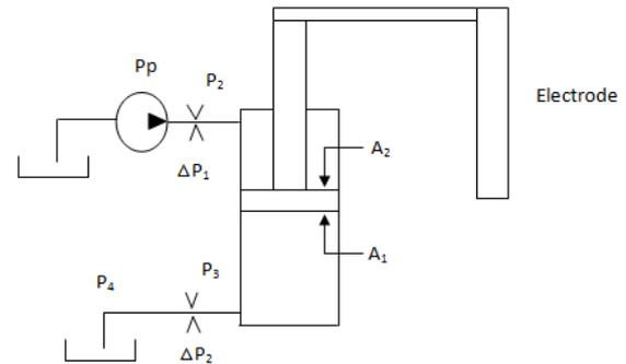
**Fig. 4. Circuit diagram of potential overrunning load.**
