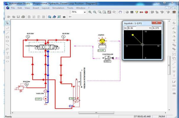
Fig. 5. The simulation in Automation Studio.
