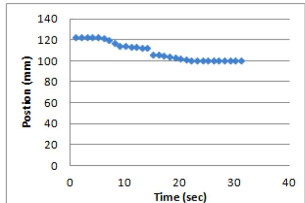
Fig. 8. Variation of cylinder position with value input signal.
