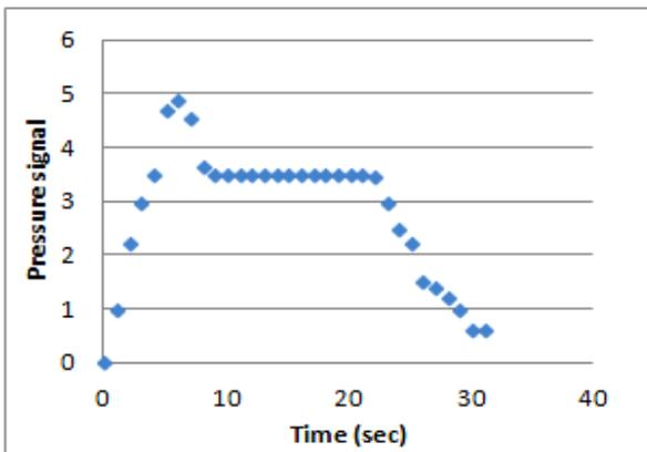
Fig . 11. Variation of pressure of hydraulic system with input signal.
