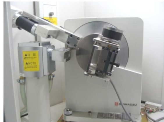
Fig. 2. X-ray stress analyzer (XRD-6000) used to measure the residual stresses.
