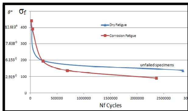
**Fig. 5. Conventional ,constant stress amplitude S-N curves for dry and corrosion fatigue conditions.**
