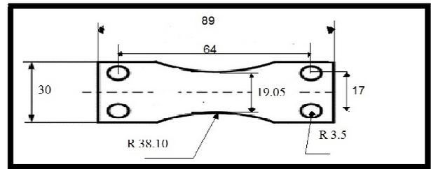
Fig. 3. Shape and dimensions of fatigue specimen ( all dimensions in mm) according to ASTM D3479/D3479M-96 standard
