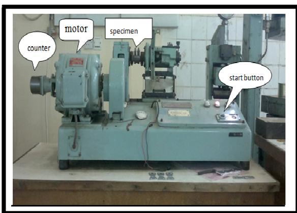
Fig. 2. Fatigue testing machine.
