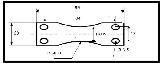
Fig. 3. Shape and dimensions of fatigue specimen ( all dimensions in mm) according to ASTM D3479/D3479M-96 standard
