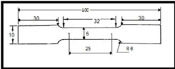
Fig.1. Tensile test specimen according to ASTM B209.
