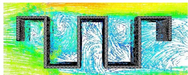
Fig. 16. Velocity Distribution Around Rectangular Extended Surface.
