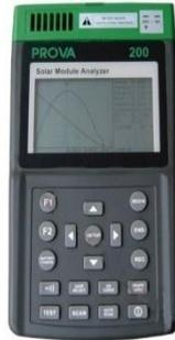
Fig. 5. The Prova 200 solar panel analyzer.
