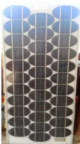
Fig. 2. Monocrystalline panel.
