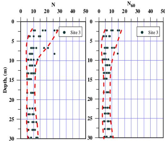
Fig. 15. Standard Penetration Test Results for Site 3.
