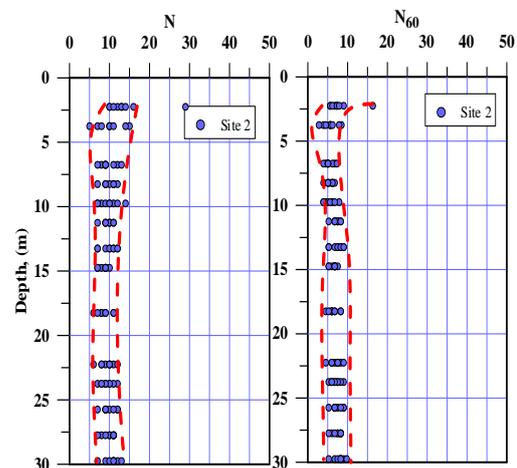
Fig. 14. Standard Penetration Test Results for Site 2.
