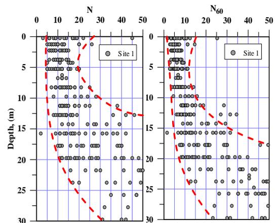
Fig. 13. Standard Penetration Test Results for Site 1.
