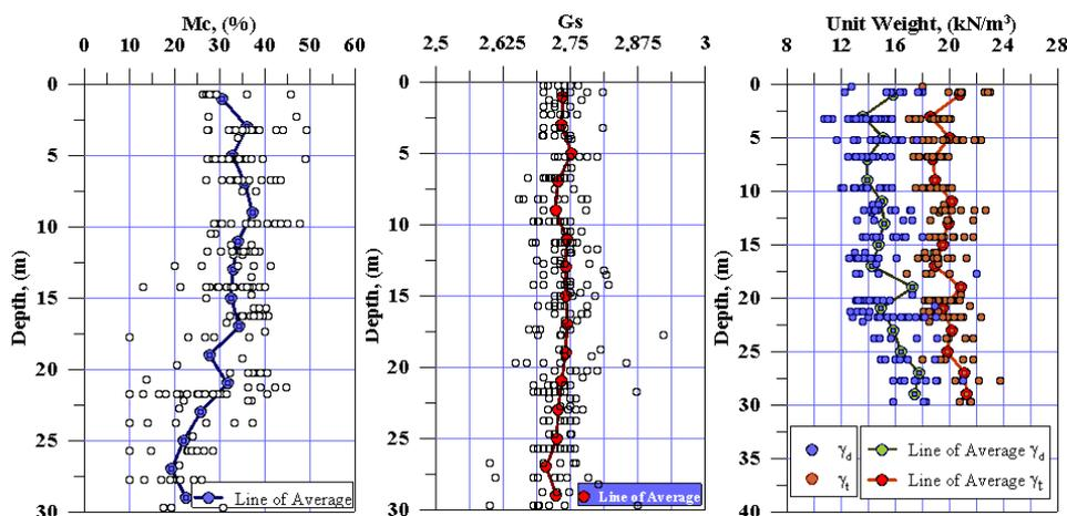
**Fig. 5. Variation of Moisture Content, Specific Gravity and Bulk Unit Weight of Basra Soil.**
