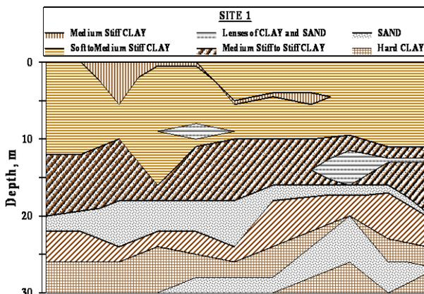
Fig. 16. Typical profiles for Site 1.
