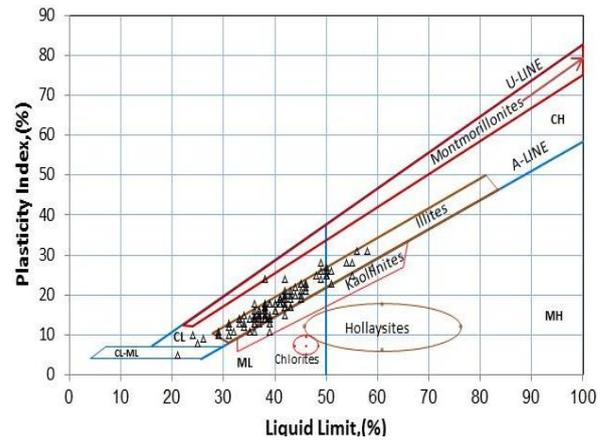
Fig. 9. Plasticity Characteristics of Common Clay Minerals.
