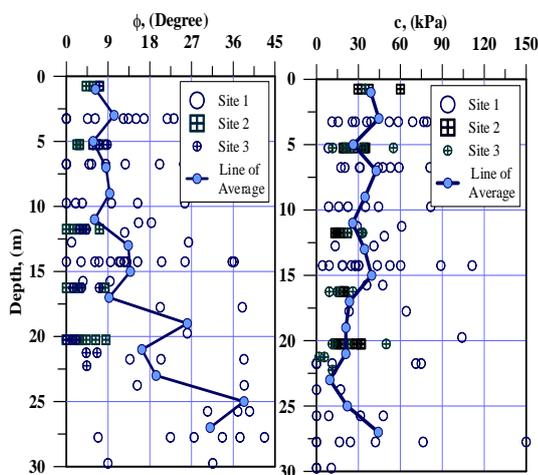
Fig. 12. Variation of Direct Shear Test Results of Basra Soil
