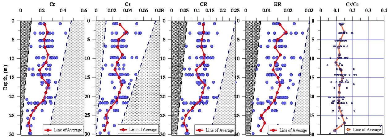
Fig. 10. Consolidation Parameters of Basra Soil.
