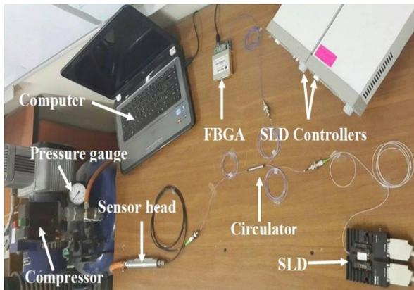
Fig. 3. Experimental setup.
