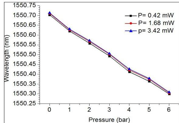
Fig. 6. Bragg wavelength shift against pressure at different sets of powers.
