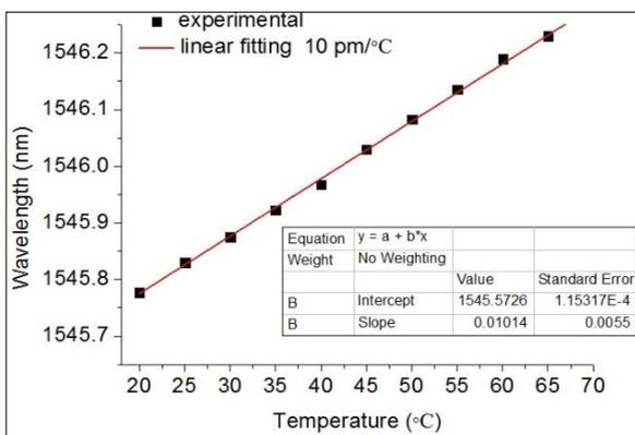
**Fig. 8. First peak shift (FGB1) with temperature increased.**
