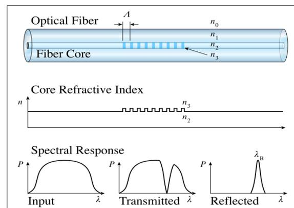
**Fig. 1. Structure of FBG and the reflection and transmission spectrum [4].**
