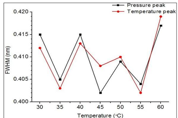
**Fig. 10. FWHM change with temperature increased for FBG1 and FBG2.**
