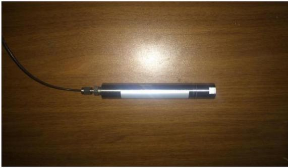
Fig. 2. FBG sensor head.
