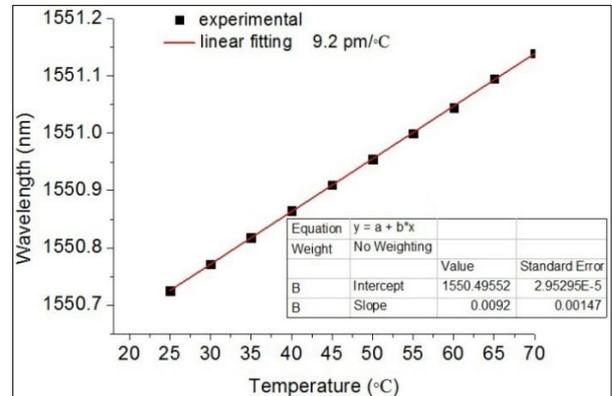
**Fig. 9. Second peak shift (FBG2) with temperature increased.**
