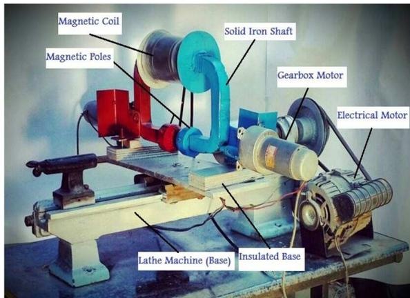
**Fig. 3. Photograph of the MAF Machine.**
