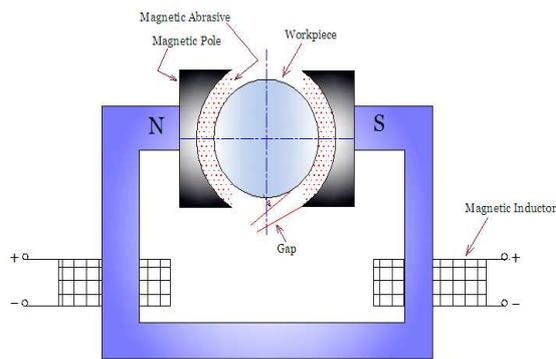
Fig. 1. Scheme of magnetic abrasive finishing (MAF): External finishing.
