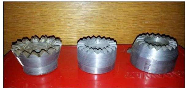
**Fig. 4. The three manufactured magnetic poles.**
