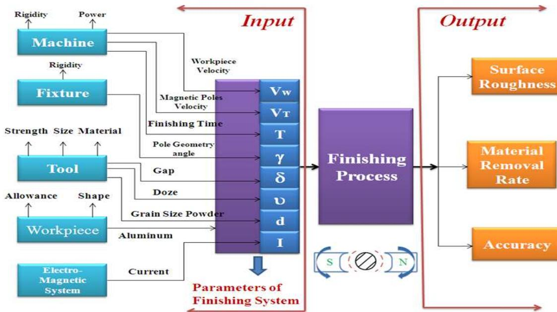
Fig. 2. Input and output for the Finishing System for MAF.
