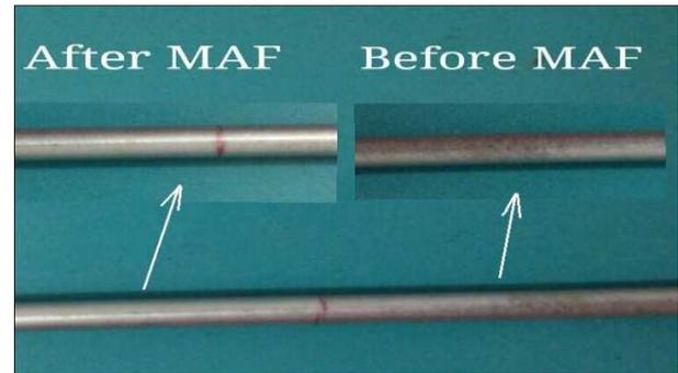
Fig. 5. Duralumin workpiece before after MAF process.
