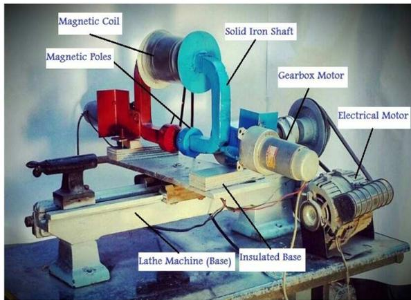
**Fig. 3. Photograph of the MAF Machine.**
