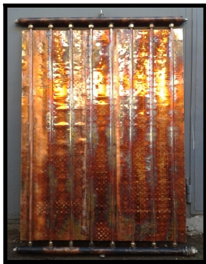
Fig. 3. copper sheet welding to the riser pipes.
