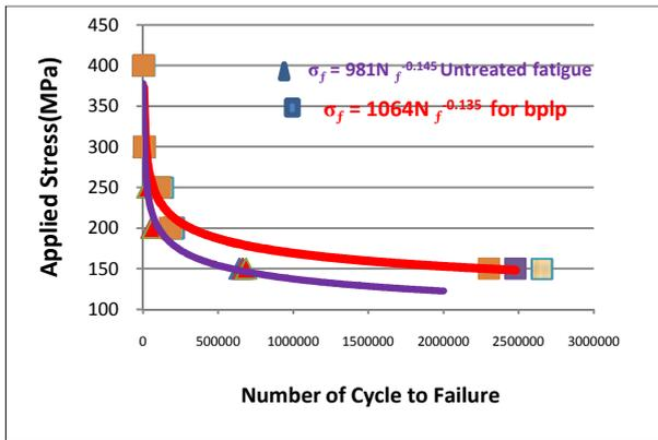
Fig. 5. Conventional basic line S-N curve for untreated and bplp fatigue .
