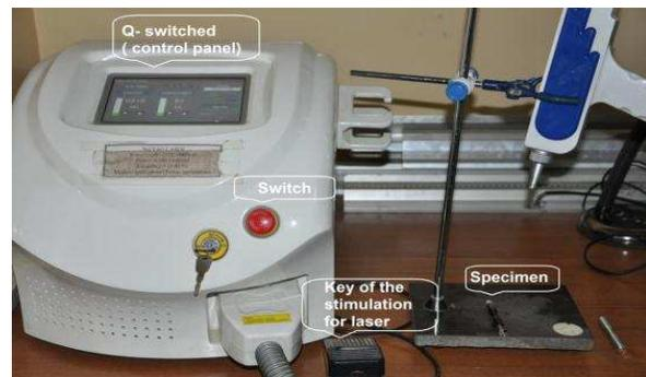
Fig. 3. Nd-YAG laser peening device at university of Technology-Baghdad .
