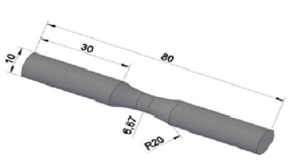
Fig. 1. Fatigue specimen dimensions (DIN 50113) (all dimnsions in mm).
