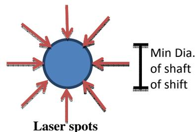
Fig. 4. Laser spots around min. diameter of fatigue specimen.
