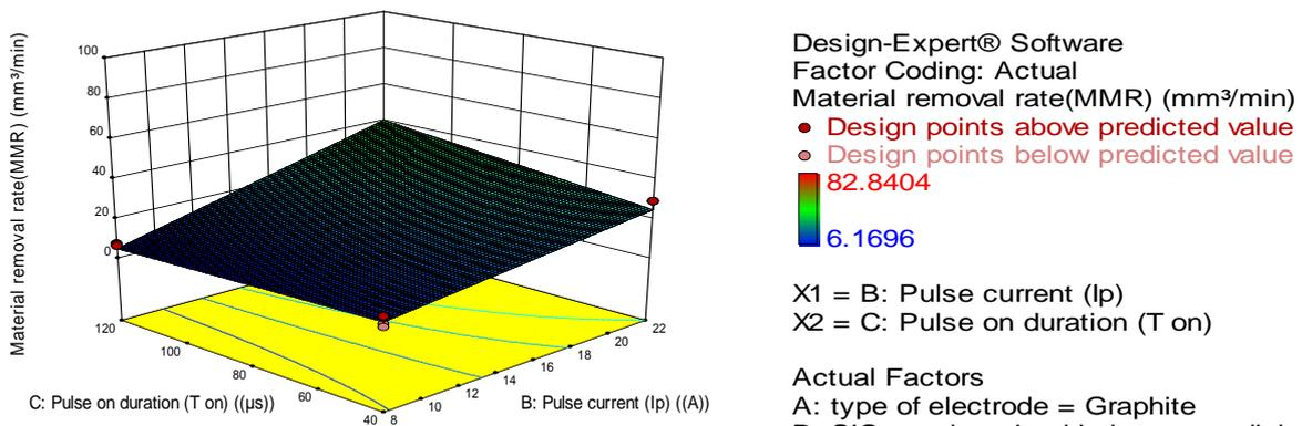
**Fig. 4.** The 3D graphs for MRR using kerosene dielectric alone and the graphite electrodes.
