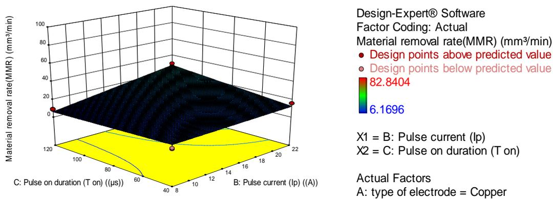
**Fig. 3.** The 3D graphs for MRR using kerosene dielectric alone and copper electrodes
