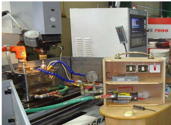
Fig. 2. The (CNC) EDM machine with all the manufactured accessories designed for the implementation the PMEDM experiments.
