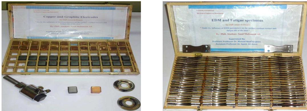
Fig. 1. The copper and graphite electrodes and workpieces PMEDM processes.
