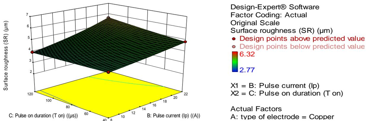
**Fig. 11.** The 3D graphs for SR using the copper electrodes and kerosene dielectric alone.
