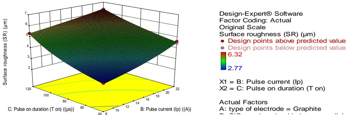
Fig. 14. The 3D graphs for SR using the the graphite and (5g/l) graphite powder mixing in kerosene dielectric.
