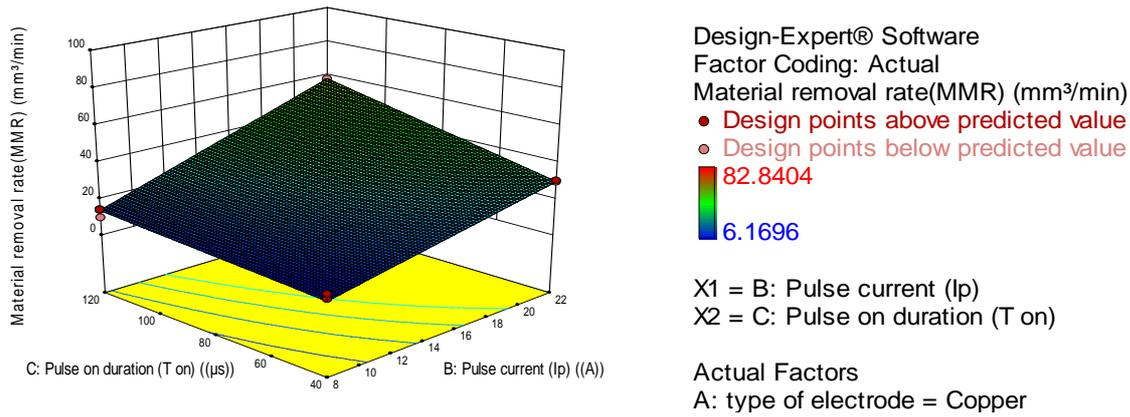
Fig. 5. The 3D graphs for MRR using kerosene dielectric with graphite powder mixing (PMEDM) and the copper electrodes.
