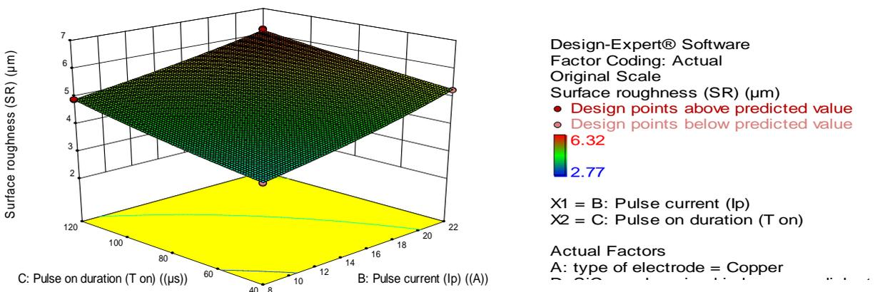
**Fig. 12.** The 3D graphs for SR using the copper electrodes and (5g/l) graphite powder mixing in kerosene dielectric
