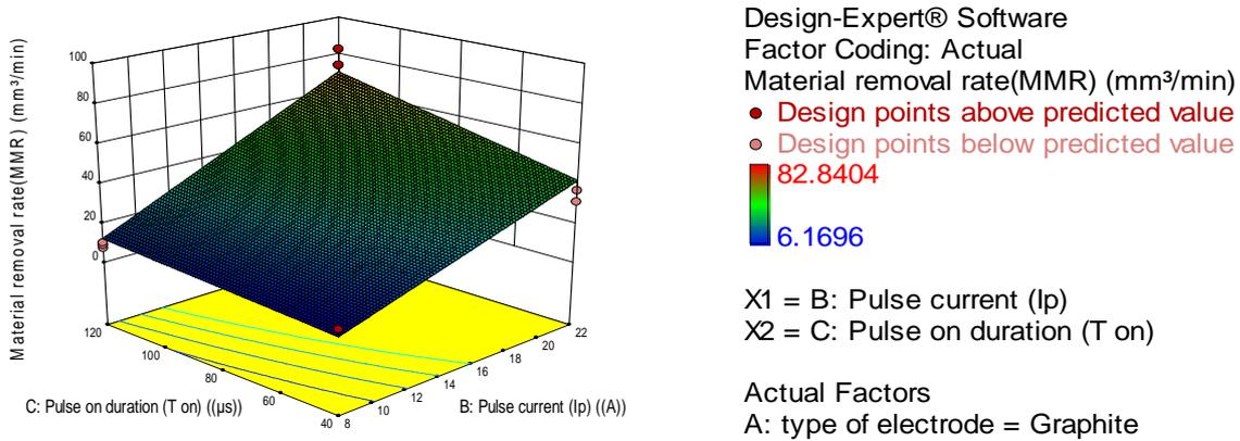
Fig. 6. The 3D graphs for MRR using kerosene dielectric with graphite powder mixing (PMEDM) and the graphite electrodes.
