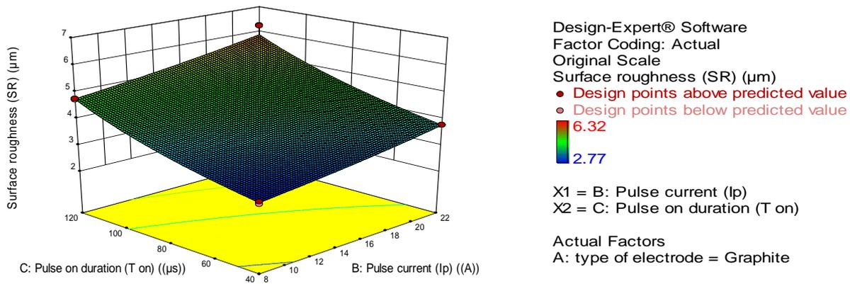
Fig. 13. The 3D graphs for SR using the graphite electrodes and kerosene dielectric alone.
