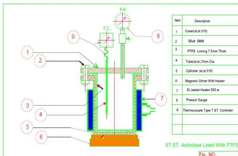
Fig. 1. Twin autoclaves lined with PTFE.
