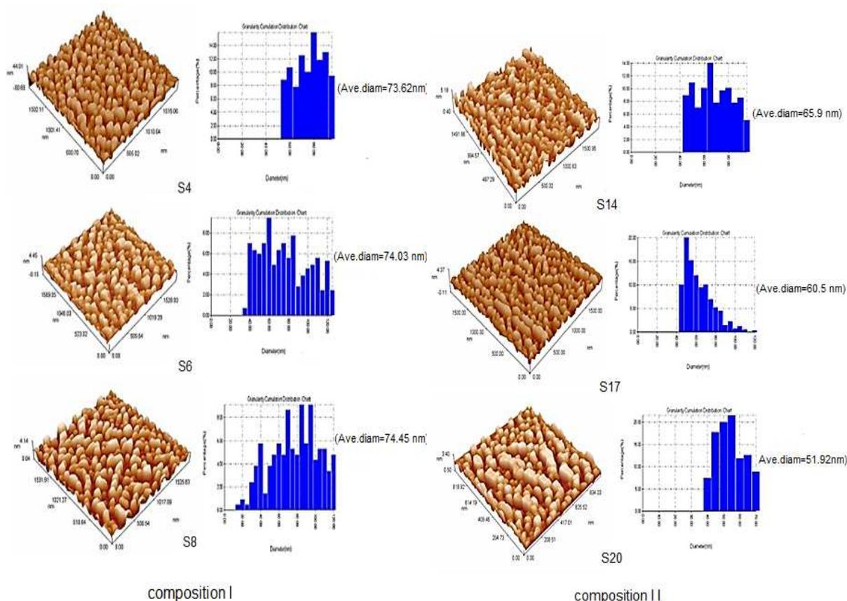
Fig. 4. Atomic force microscopy reports for samples of composition I & II.
