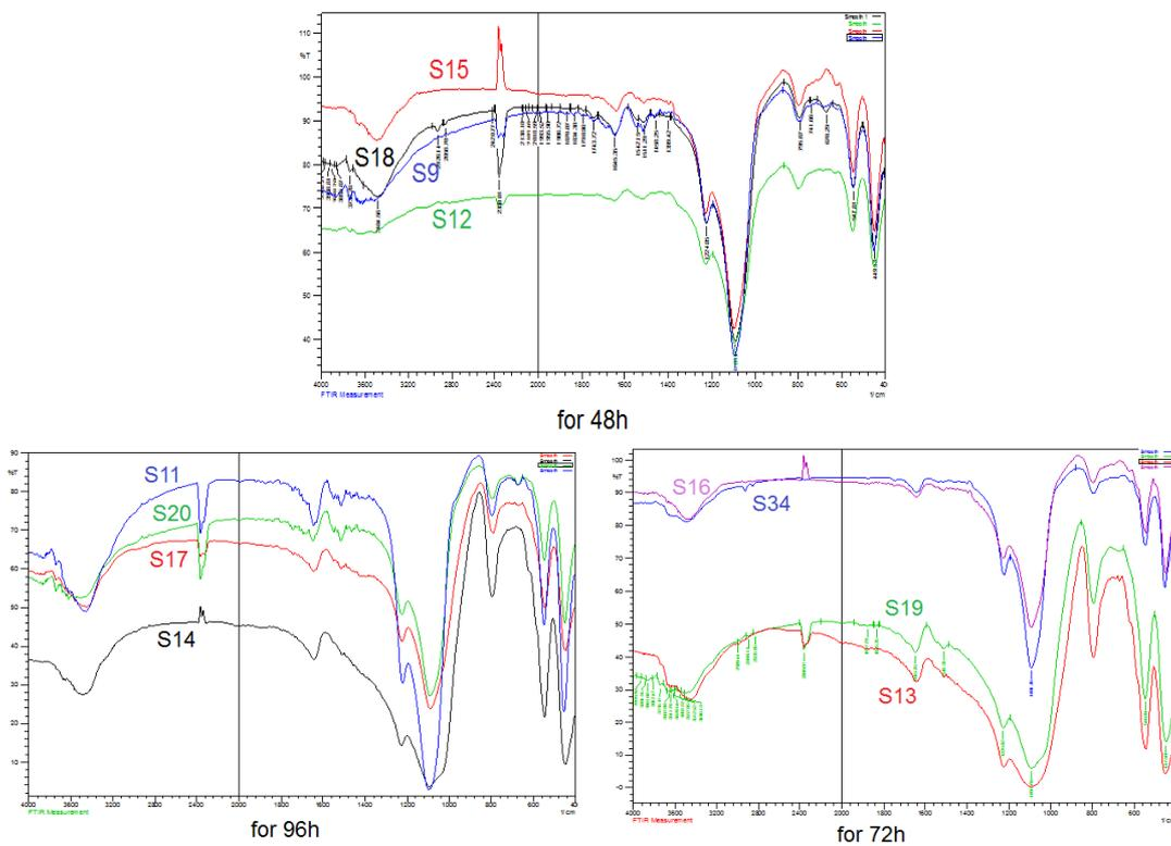
Fig. 7. FTIR spectra for the samples prepared at various crystallization time (96h,72h,48h) and temperatures of (180,170,160 and 150 C).
