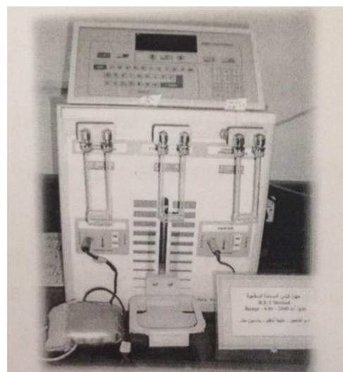
Fig. 2. BET surface area analyzer.
