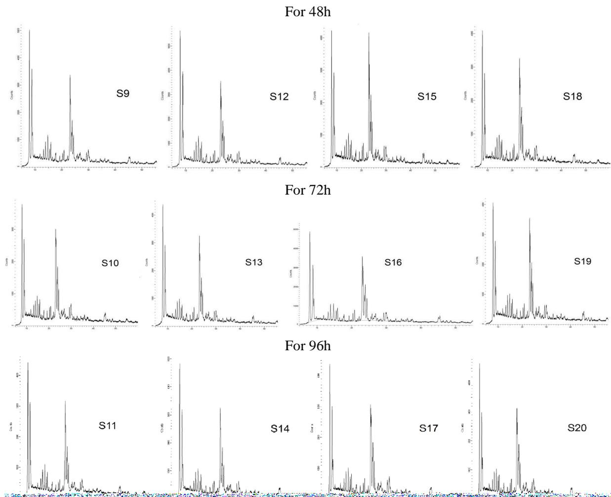
**Fig. 5.** XRD patterns at different crystallization temperatures (150,160,170 and 180 C) for different crystallization times (48,72,and 96h).
