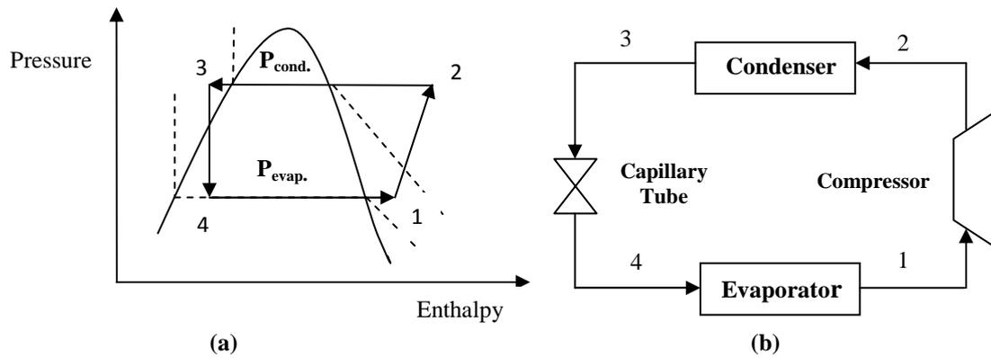
Fig. 3b.(a) Shows the process path on a pressure–enthalpy (P– h) diagram, and (b)shows a schematic diagram of the process equipment.
