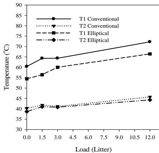
Fig. 4. Variation the Inlet and Outlet Temperature of the Condenser with Load.
