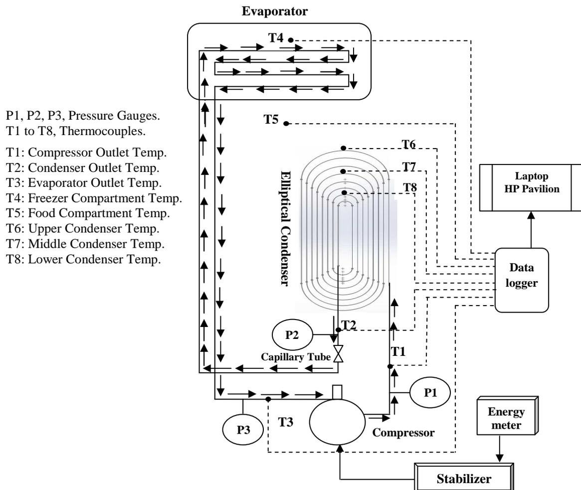
Fig. 3a. Schematic Diagram of the Investigation Unit and Apparatus.
