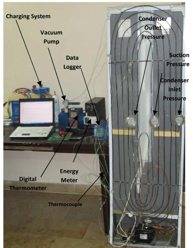
Fig. 2. Experimental Setup of the Investigation Unit and Apparatus.
