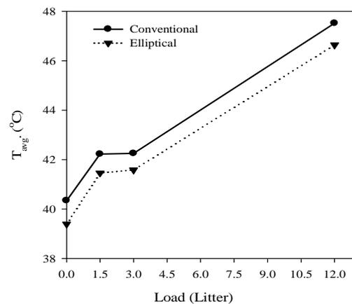
Fig. 5. Variation of the Average Temperature at the Surface of the Condenser (T6,T7 and T8) with Load.
