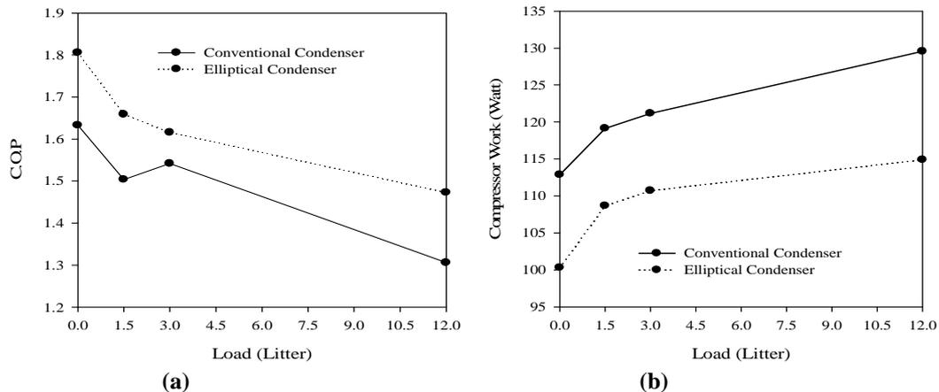
Fig. 8 (a) variation the coefficient of performance and (b) the compressor work with all load.
