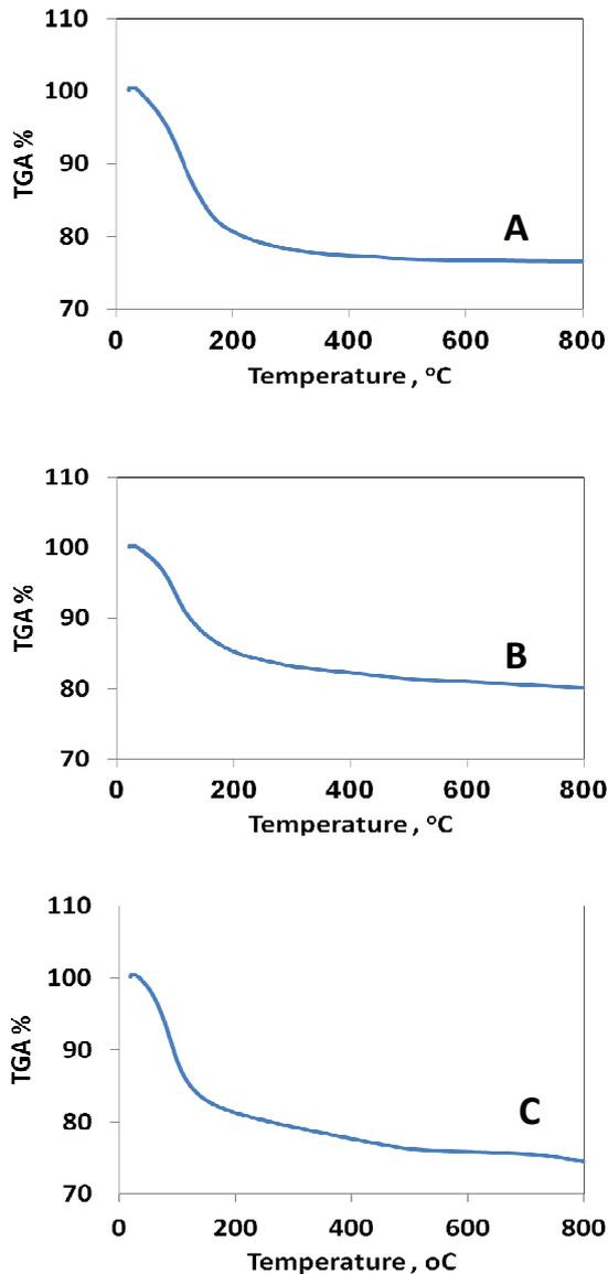
Fig. 6. TGA of Zeolite Y, (A) Synthesized NaY, (B) Synthesized HY, (C) Commercial HY.
