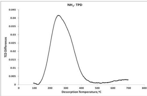
Fig. 10. NH<sub>3</sub>-TPD of prepared NaY zeolite.
