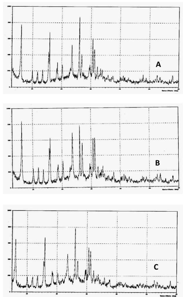
**Fig. 2. XRD pattern of synthesis Na- Y zeolite at different aging time (A. 24 hr. , B. 48 hr., C. 72 hr.), X-axis 2theta,Y-axis Intensity .**
