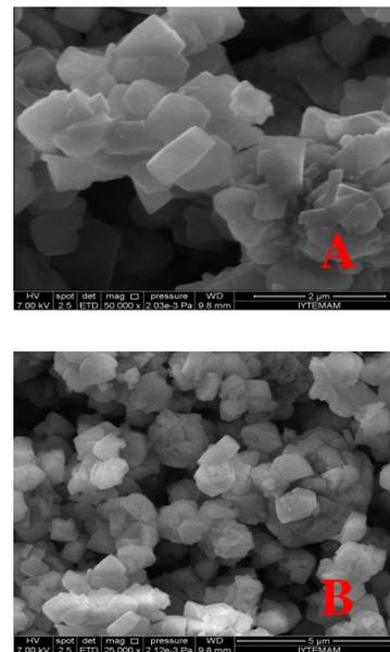
Fig. 8. SEM images of commercial zeolite Y, (A)25 000 X, (B) 50 000 X.
