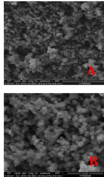
Fig. 7. SEM images of Synthesized zeolite Y, (A)25 000 X, (B) 50 000 X.
