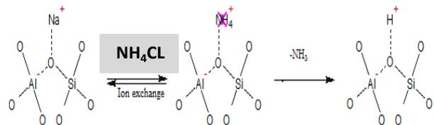
Fig. 4. Ion-exchange of Na-form of zeolite Y into H-form zeolite.
