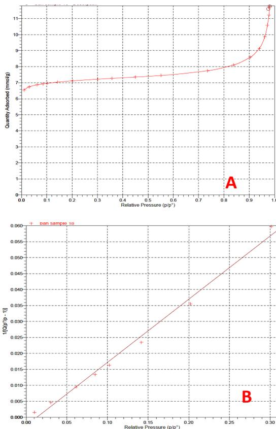
Fig. 3. (A) Adsorption Isotherm of prepared Y zeolite at aging time 48hr, (B) BET plot.
