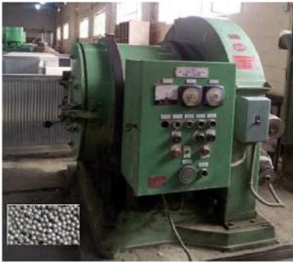
Fig. 2. Shot Peening Device with shot balls.
