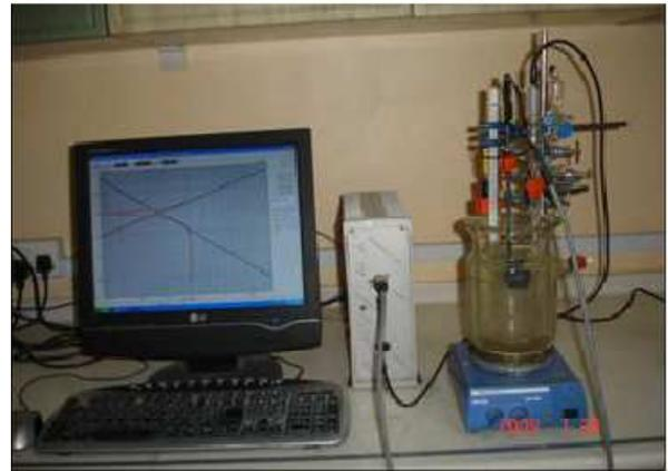
**Fig. 4. The electrochemical corrosion unit.**
