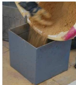
Required amount of expansive soil is poured onto the soil container
