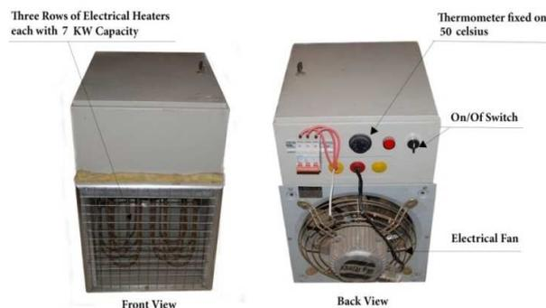
Fig. 5. Heating Duct Details.
