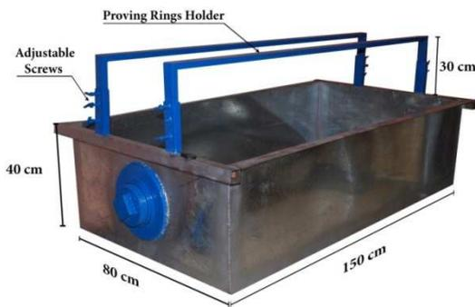
Fig. 7. Saturation-drying tank for pile uplift force measurement.
