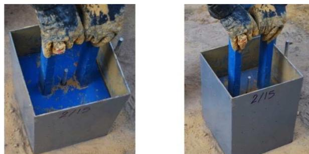
Compaction of soil to the required level by using the specially manufactured hand hammer
