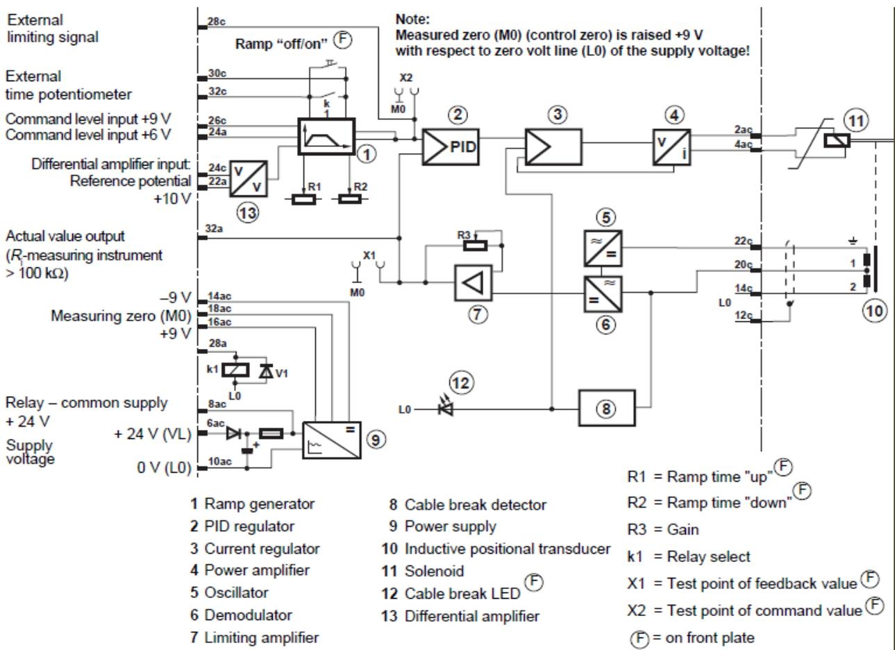
Fig. 5. Terminal Connections / Block Circuit Diagram Electronic control: Amplifiers Model VT 5010 for velocity control [15].
