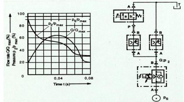
Fig. 8. Step response of a flow control valve to a step load [16].
