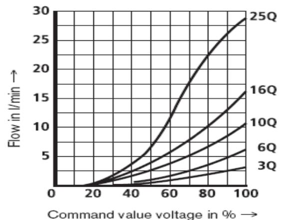
**Fig. 10. Dependency flow rate on signal value voltage for different valve size [15].**
