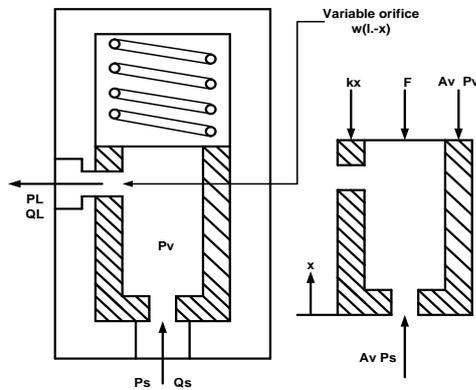
Fig. 1. Schematic of physical analysis of flow control valves.
