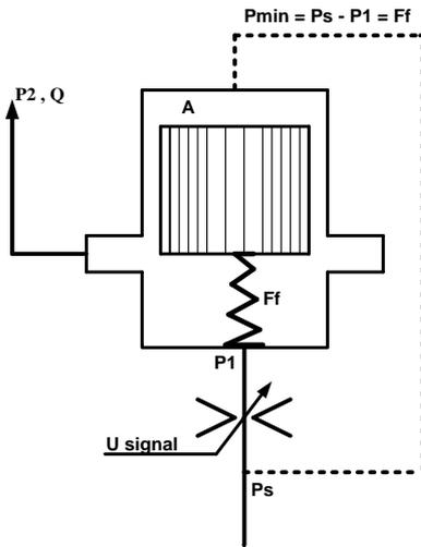
Fig. 6. Model of a 2-way proportional flow control valve.
