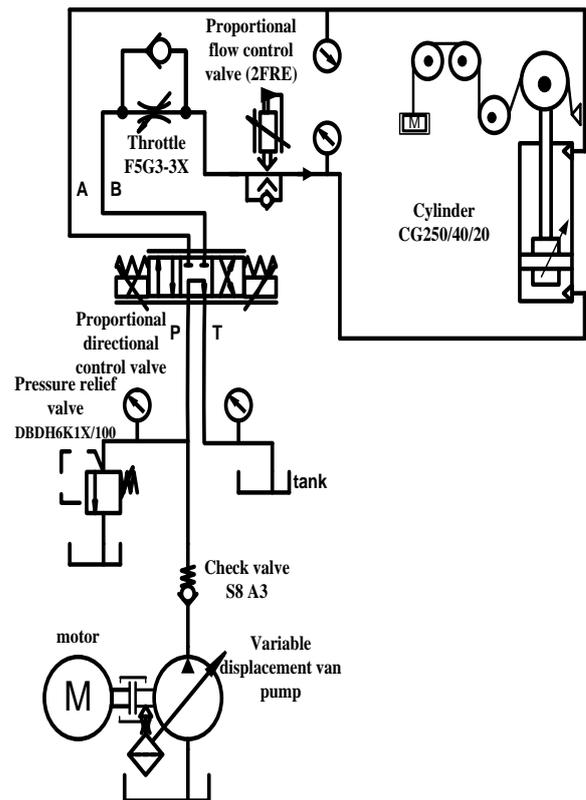
Fig. 4. Schematic diagram of connection Electro-hydraulic control circuit.
