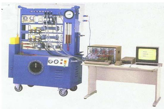
Fig. 3. Photograph of electro- hydraulic control unit test bench [15].
