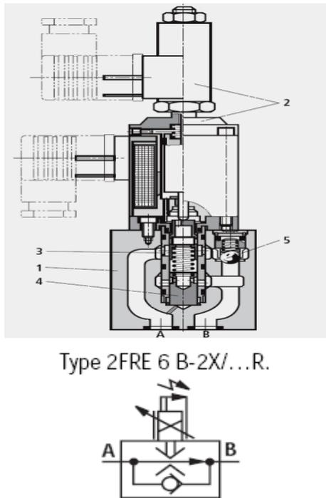
Fig. 2. Proportional flow control valve 2FRE 6 B-2X/...4RV [15].
