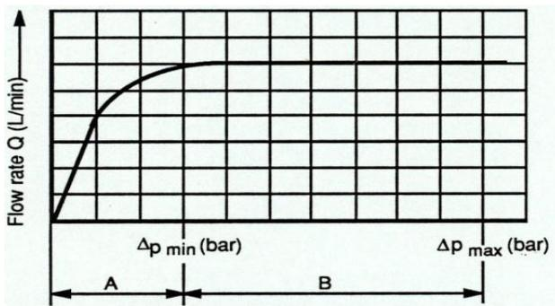
Fig. 7. Qualitative characteristic curve of a flow control valve [16].
