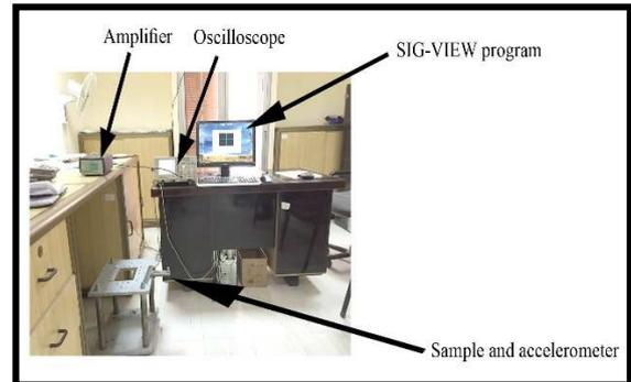
Fig. 3. Damping test setup with assembled sample.
