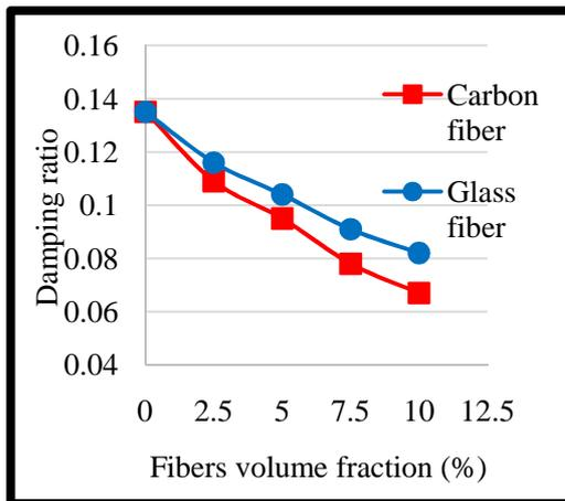
Fig. 11. Effect of fibers volume fraction on damping ratio.
