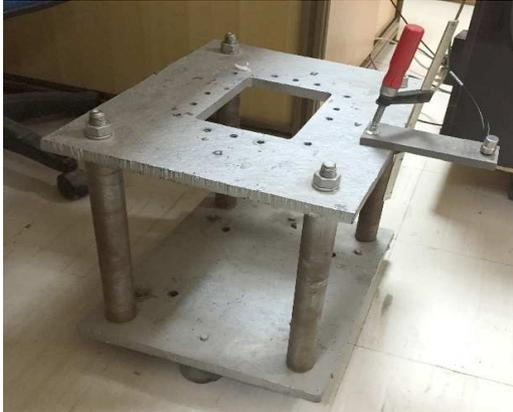
Fig. 9. The setup of the specimen for damping test.
