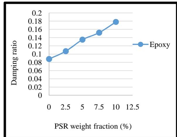
Fig. 10. Effect of PSR weight fraction on damping ratio.
