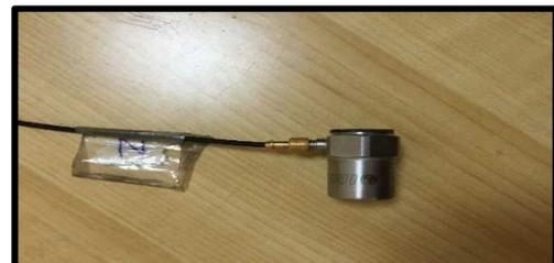
Fig. 5. The accelerometer.
