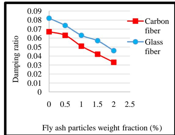
Fig. 13. Effect fly ash particles weight fraction on damping ratio.
