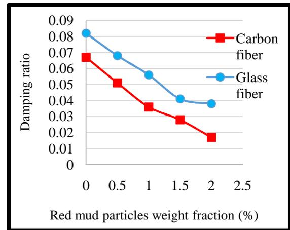
Fig. 12. Effect of red mud particles weight fraction on damping ratio.
