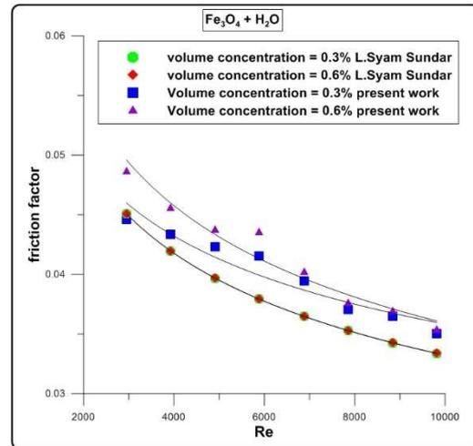
Fig. 8. Comparison of experimental data of the present work with the L.Syam Sundar, the effect of Reynold on friction factor.
