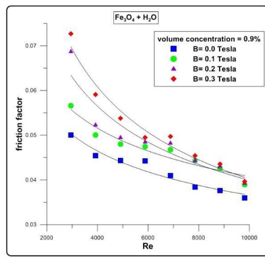
Fig. 10. The effect of Reynolds number on friction factor with different magnets.
