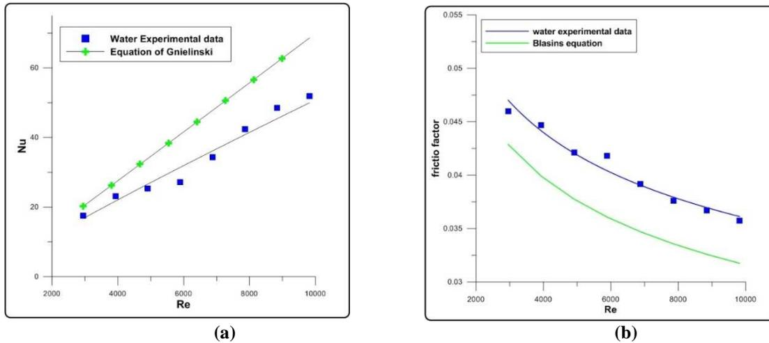
Fig. 2. (a) The effect of Reynolds number on Nusselt number for distilled water with Gnielinski’s equation, (b) The effect of Reynolds number on friction for distilled water with Blasius equation.
