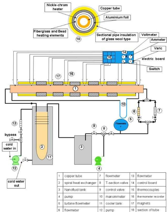
**Fig.1. Schematic diagram of the experimental test rig.**
