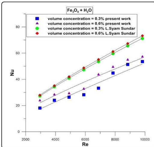
Fig. 7. Comparison of experimental data of the present work with the L.Syam Sundar, the effect of Reynold on Nusselt number.
