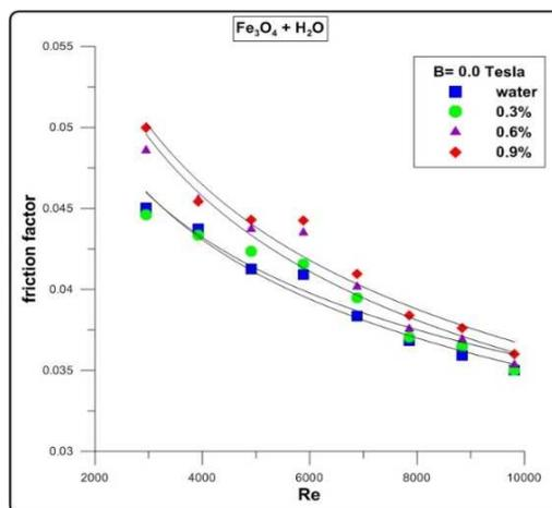
Fig. 9. The effect of Reynolds number on friction factor.
