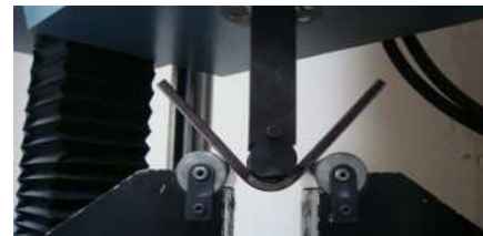
Fig. 7. Bending Setup (Push travel technique).
