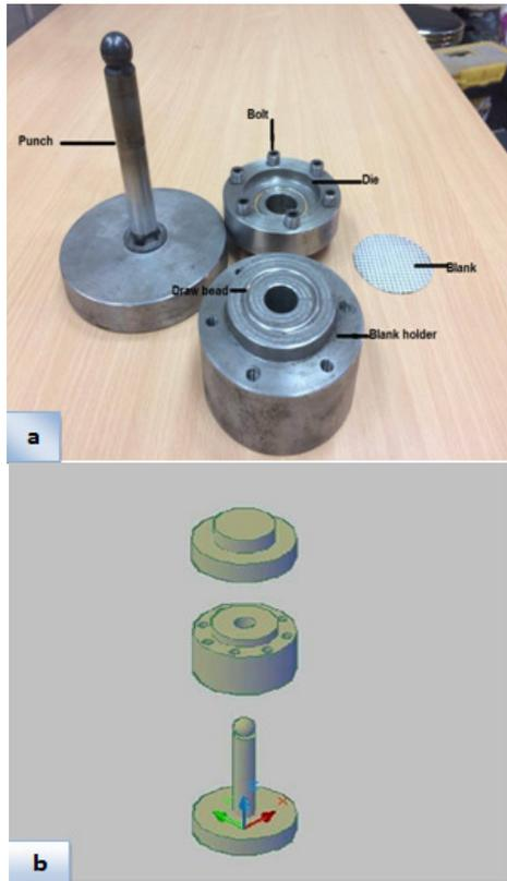
Fig. 4. Stretching forming equipments used. a) physical tools representation, b) assembly view representation.
