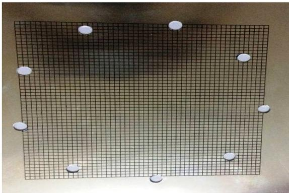
Fig. 9. Sheet metal with square grid.
