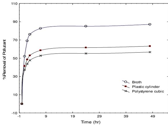
Fig. 15. Effect of Packing type on the Removal percent of TOC pollutant with time at T=25°C, pH 7, and sterilized wastewater.
