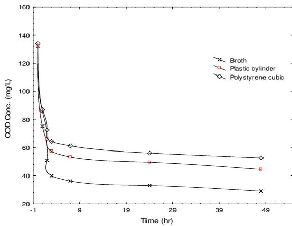
Fig. 16. Effect of Packing type on the concentration level of COD pollutant with time at T=25°C, pH 7, and sterilized wastewater.
