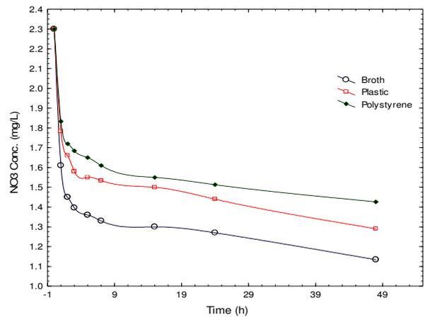
Fig. 18. Effect of Packing type on the concentration level of NO<sub>3</sub> pollutant with time at T=25°C, pH 7, and sterilized wastewater.
