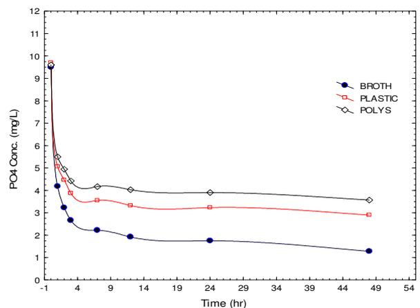
Fig. 20. Effect of Packing type on the concentration level of PO<sub>4</sub> pollutant with time at T=25°C, pH 7, and sterilized wastewater.
