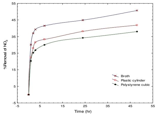
Fig. 19. Effect of Packing type on the Removal percent of NO<sub>3</sub> pollutant with time at T=25°C, pH 7, and sterilized wastewater.
