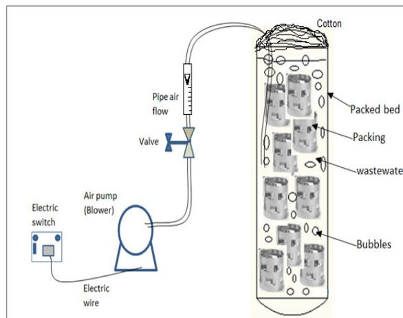
**Fig. 1. Process flow diagram of the wastewater treatment by microalgae.**
