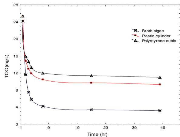
Fig. 14. Effect of Packing type on the concentration level of TOC pollutant with time at T=25°C, pH 7, and sterilized wastewater.
