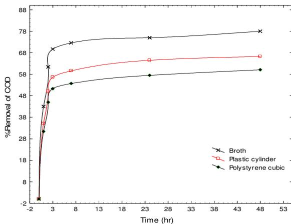
Fig. 17. Effect of Packing type on the Removal percent of COD pollutant with time at T=25°C, pH7, and sterilized wastewater.
