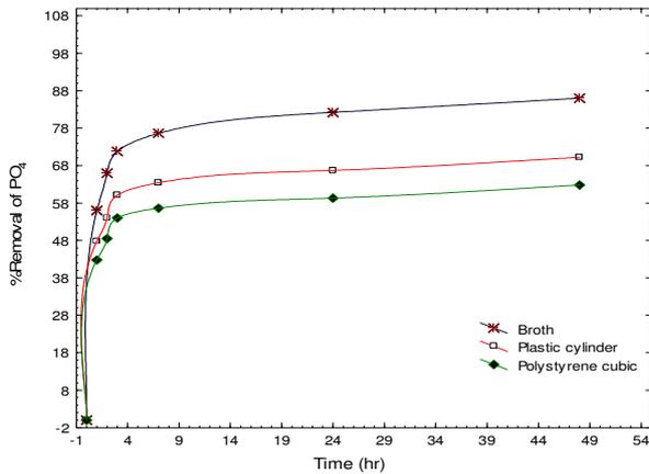
**Fig. 21. Effect of Packing type on the Removal percent of PO<sub>4</sub> pollutant with time at T=25°C, pH7, wastewater/ (Algae packing) ratio =1, and sterilized wastewater.**
